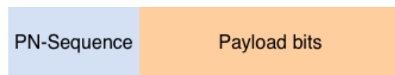
Figure 4.4: Frame structure with PN-sequence preamble. The number of payload bits is arbitrary.
