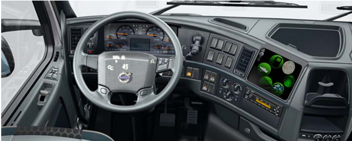
Picture 41: Showing real-time feedback on steering wheel with: pending voice message, eco cruise control activated and comparing to company average. The large display is placed to the right of the steering wheel showing the six basic icons.
