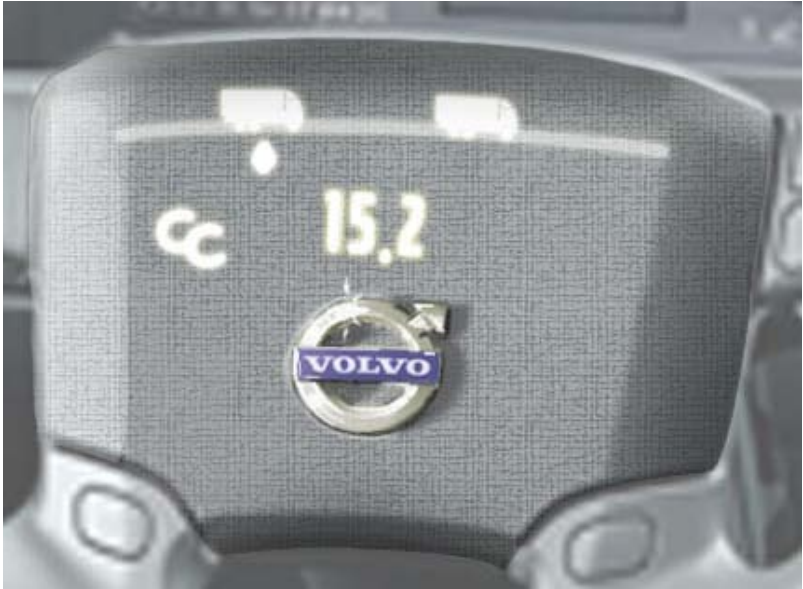
Picture 21: Eco Cruise Control is activated together with Virtual partner comparing with colleague and current fuel usage display.
