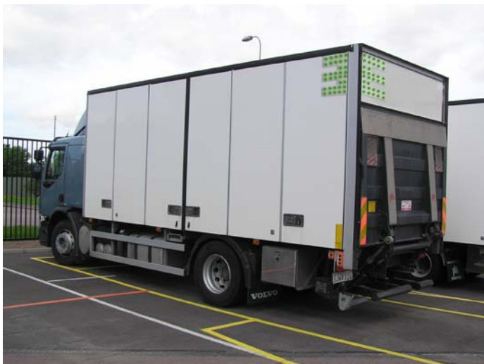
Picture 39: Green LED-lights placed on the cab exterior indicating eco-driving
