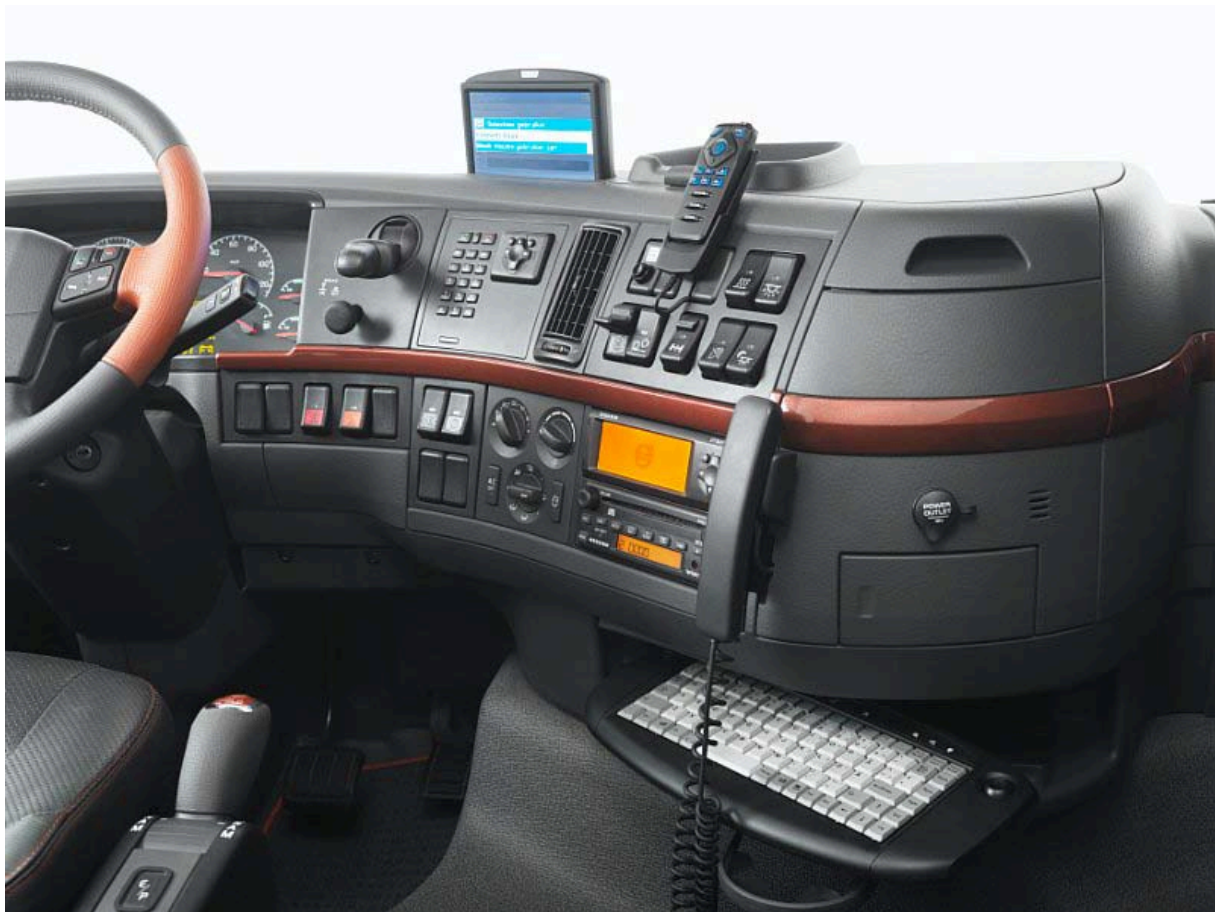
Picture 13: Dynafleet system in a truck cab, showing computer keyboard. Approved for publication by: Christer Lindqvist, Brand manager, Volvo Truck Corporation
