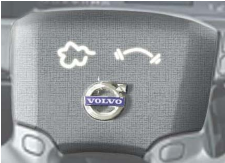
Picture 24: Real-time advice displaying from left to right: idling icon and overload icon
