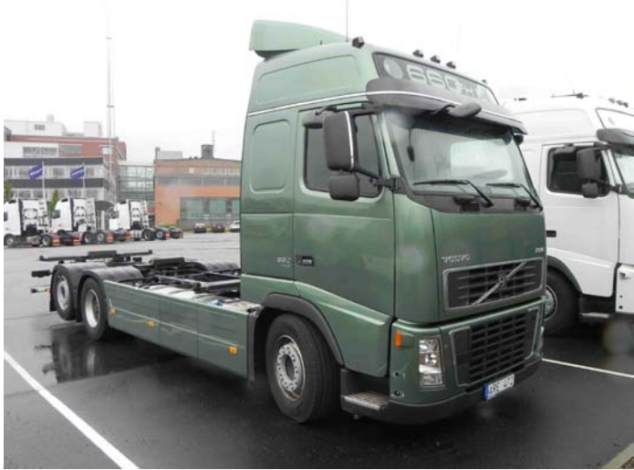
Picture 1: Towing engine/truck tractor that combines with a semi-trailer to create a semi-trailer truck. Photo: M. Ingemansson, Publication approved by Volvo Group
