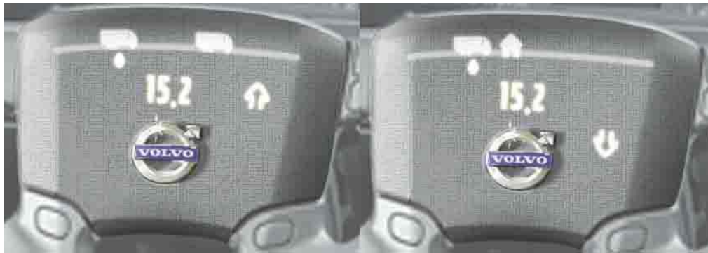
Picture 23: Accelerating and decelerating icons are lit to advise driver to take the necessary actions
