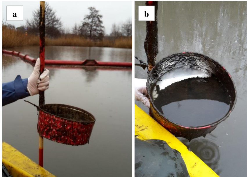
Figure 18. (a) Sediment trap after deployment; (b) Sediment trap with accumulated sediment (Björklund, 2017).
