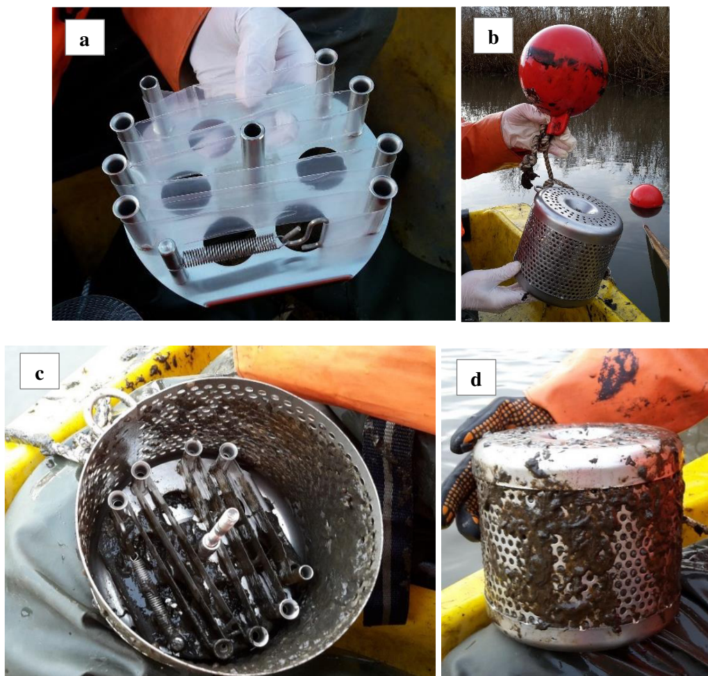
Figure 16. (a) SPMD membrane mounted on spider before deployment; (b) SPMD sampler with buoy; (c) Open protection cage after deployment; (d) Protection cage after deployment (Björklund, 2017).
