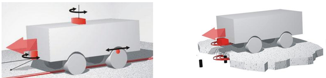
Figure 2.2 - Principle sketch for dead reckoning (left) and for magnet navigation (right) (Source: Götting KG)
