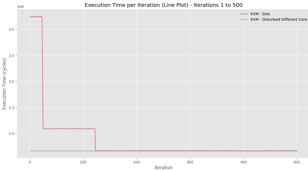
Figure 4.13: Basicmath: Line plot of the first 500 iterations of QEMU/KVM with a disturbed guest and a solo guest, showing the performance ramp-up for the solo guest.
