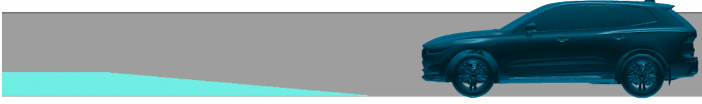
Figure 3.5: Initial volume of water present in the domain when the simulation was started, shown in turquoise. The water depth increases gradually as one progresses in front of the vehicle from zero to full wading depth. The image shows a cross section of the domain where much of the area aft of the vehicle has been cropped of.
