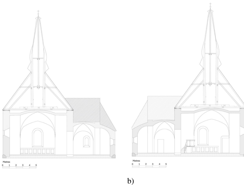
Figure 4.3: Sectional view of Skörstorp's Church a) section A north and b) section B south.
