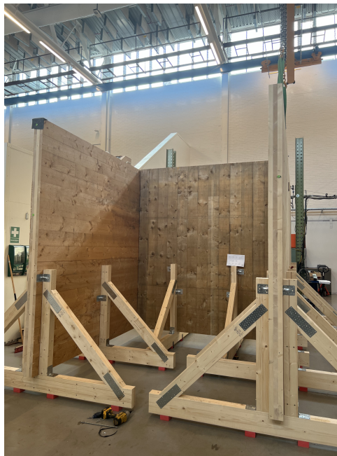
Figure 3.7: Structure without vibrational dampening material.
