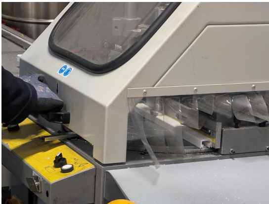
Figure 3.8: Precision abrasive saw for initial rail sectioning.
