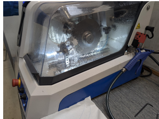
Figure 3.9: Metallographic cutting machine for cross-sectional and longitudinal slicing.
