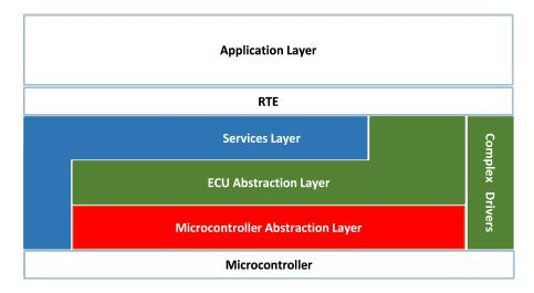
Figure 4.3: The layered AUTOSAR architecture [6]
