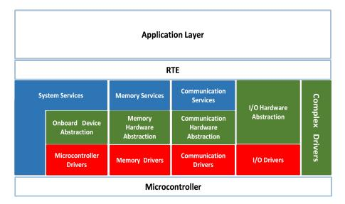
Figure 4.4: Each sub-layer of the BSW layer offers different services [6]
