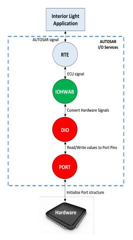
Figure 7.3: DFD diagram of the Interior light Application - I/O Layers
