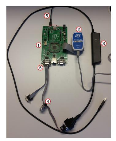
Figure 7.5: STM32 Hardware board provided by Arccore company
