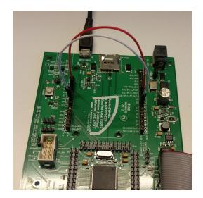
Figure 7.7: Two wires used to simulate car doors opening/closing
