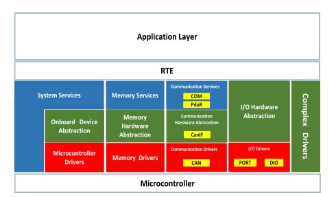
Figure 7.1: The layered AUTOSAR architecture
