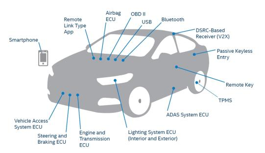
Figure 2.4: The 15 weakest points of a connected car according to Intel [124]
