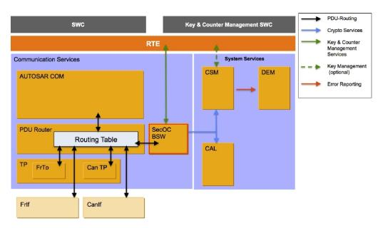
Figure 4.7: Integration of the SecOC basic software module [7]
