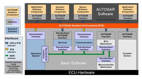
Figure 4.5: AUTOSAR software architecture - Components and Interfaces [6]
