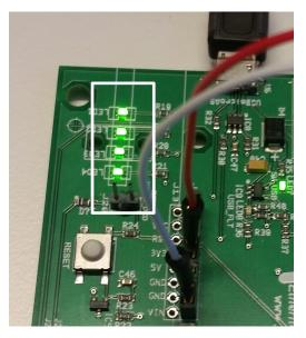
Figure 7.6: LED lights indicating if the interior light is on/off
