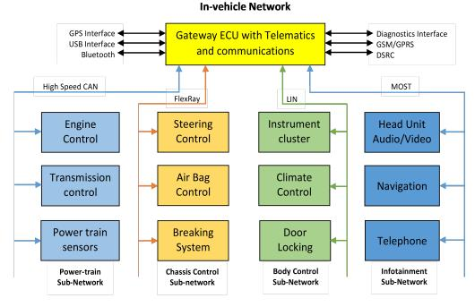
Figure 2.2: Overview of internal vehicle sub-networks [103]
