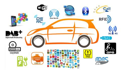
Figure 6.4: 18 most common attack surfaces of the connected car
