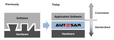
Figure 4.2: AUTOSAR hardware-independent architecture [6]
