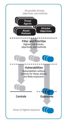
Figure 5.1: Narrowing down the field of attacks [70]
