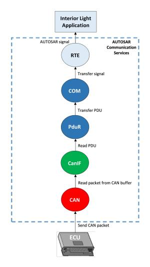
Figure 7.2: DFD diagram of the Interior light Application - COM Layers
