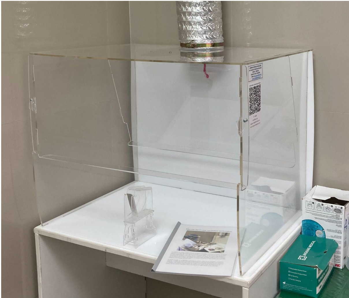
Figure 3.15 The Frugal ventilated workstation; a frugally designed ventilated workstation developed specifically for front-line AFB smear tuberculosis diagnosis.
