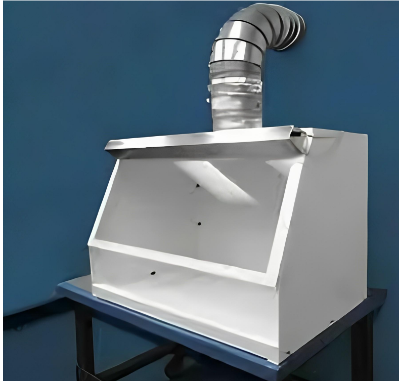
Figure 3.13 The Ventilated workstation for AFB-smear preparation (enhanced from ventilated workstation manual, CDC, 2010)
