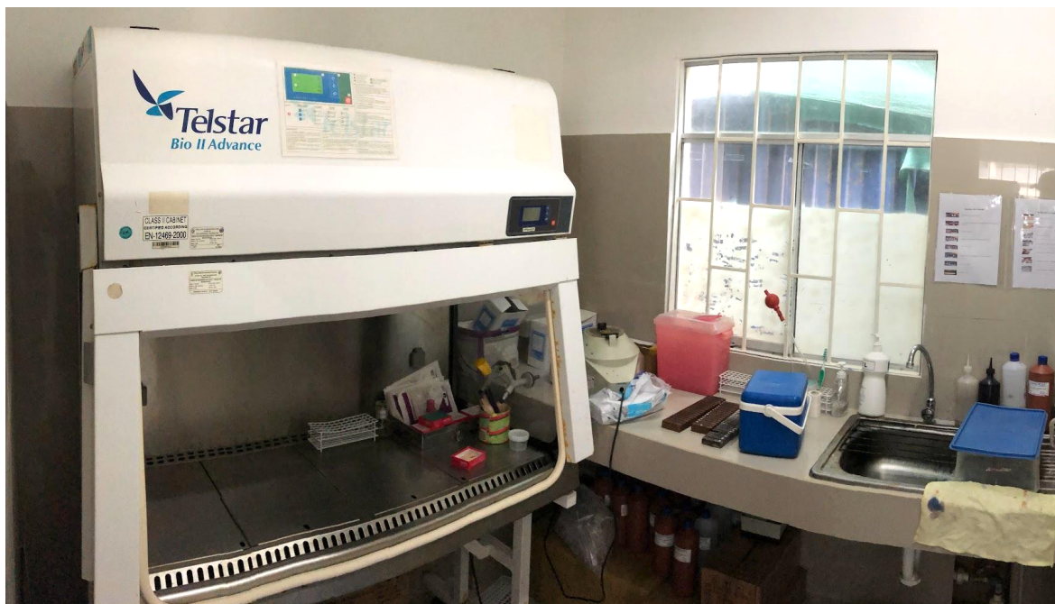
Figure 3.10 TB laboratory at National Police laboratory with a malfunctioning (Broken fan, window fallen off) BSC class II. Cost for reparation is over 10 000 USD, including technicians from US etc, according to information from laboratory technicians at the police laboratory.
