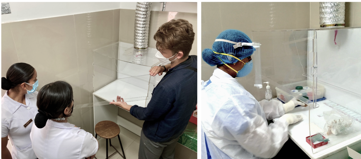
Figure 3.41 Introducing the FVWS after installation (left), first use, preparing glass slides for examination in microscopy to diagnosing sputum samples for TB (right).
