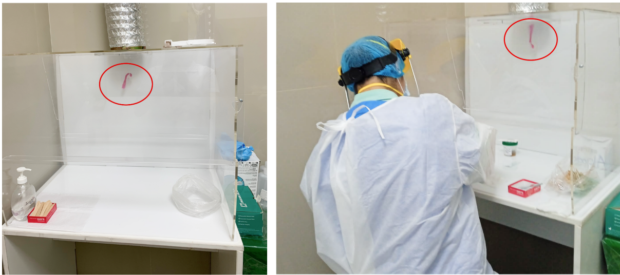
Figure 6. The yarn (circled in red) indicates if there is an airflow in the cabinet. Left: The yarn is hanging down indicating no or insufficient airflow. Right: The yarn is standing up indicating an airflow.
