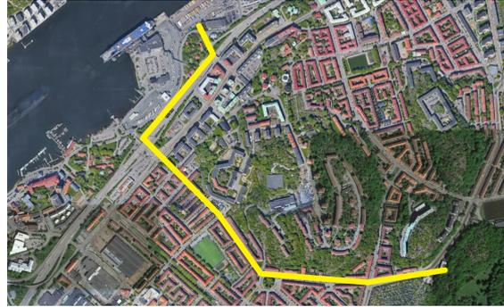
**Figure 6.2:** Demonstration for the new cable route from the 10 kV station in Slottsskogen. Map data is provided by Imagery ©2021 Aerodata International Surveys, CNES / Airbus, Landsat / Copernicus, Lantmäteriet/Metria, Maxar Technologies, Map data ©2021.
