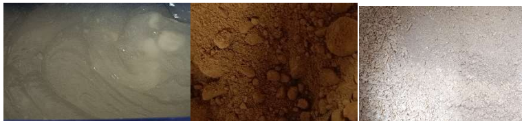
Figure 3.1: The materials used for the binder a) Wallpaper paste b) Lignin powder c) Sawdust
