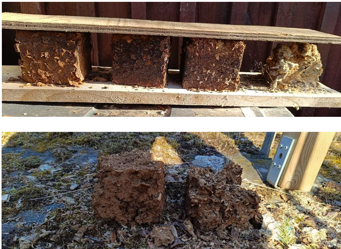
Figure IV.1: Exposure test specimen after 10 months.
