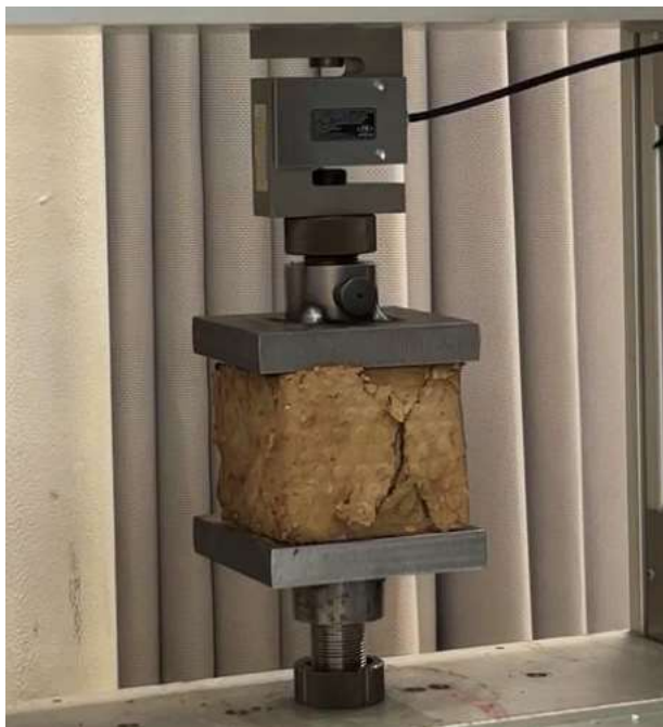
Figure 4.1: Compression failure of SLL test cube
