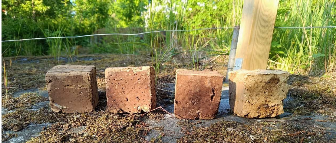
Figure 3.5: Unsheltered specimen. From left to right LLL, SLL, SSL and SSS.
