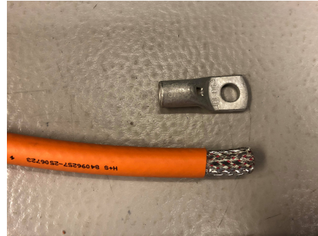
(a) Preparing test cable and cable socket. (b) Cut off the sheath until the shield.
