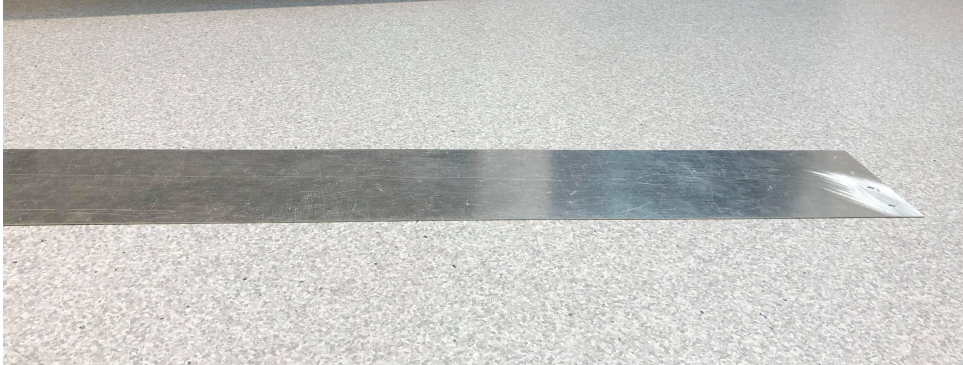
Figure 2.4: Ground reference plane for the test set-up made of a long aluminum sheet.
