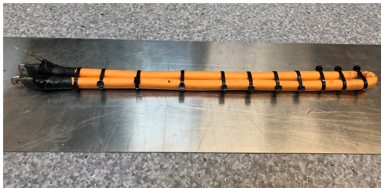
Figure 5.4: A 50 \text{mm}^2 test cable that is bent as U-shape placed on ground reference plane.
