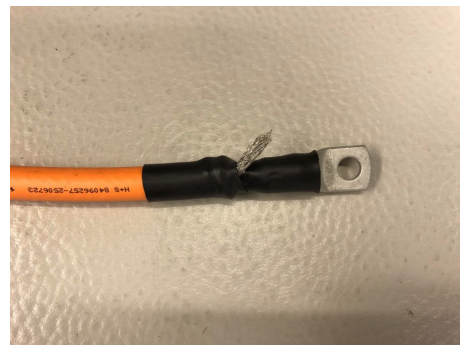
(e) Insert the conductor into the cable socket and press it. (f) Tape around the cutting area to separate conductor and shield.
