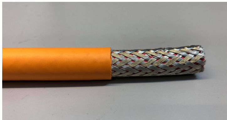
Figure 2.3: Test cable with braided shield.
