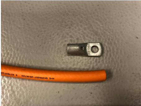
(a) Preparing test cable and cable socket. (b) Cut off the sheath until the shield.
