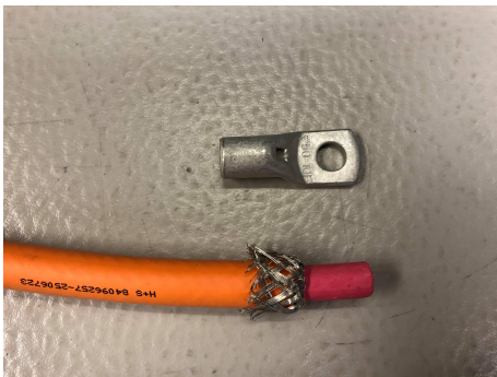
(c) Unroll the braided shield and pull it back. (d) Cut off the insulator that surrounds the conductor.
