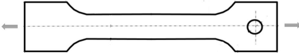
Figure 4.2: Schematic representation of Uniaxial tension test [30]
