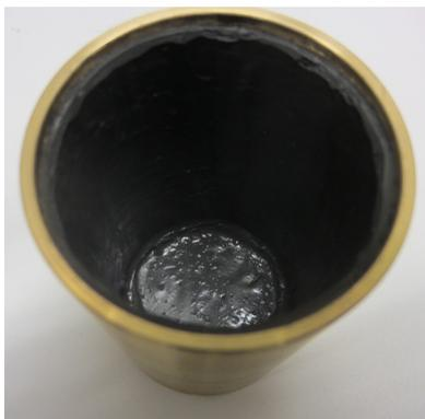
Figure 3.9: The cylinder shield painted with ECCOSORB 300.
