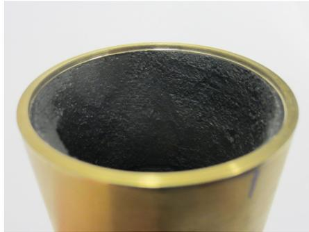
Figure 3.10: The Cylindrical shield painted with the Magic Mix "Black Hole", mixed according to table 3.1.
