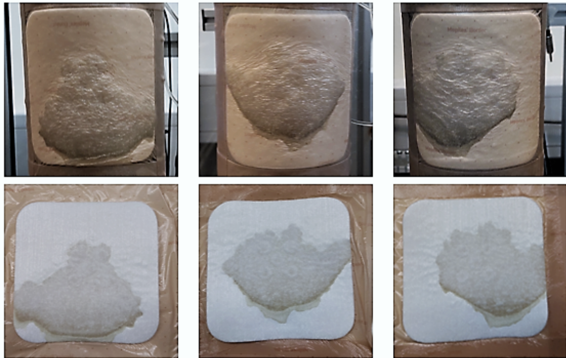
Figure 4.17: Spreading behavior of SWF C in FLUHTE, where the top row shows the back of the dressing and the bottom row shows the front of it.
