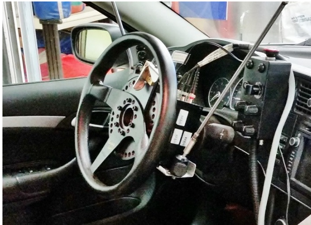
Figure 3.10: RMS FEL20 torque-measuring steering wheel installed in test vehicle
