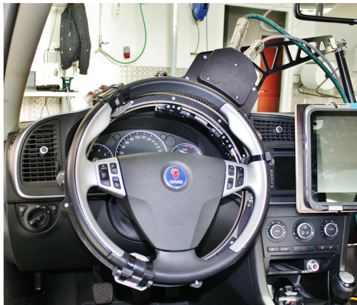
Figure 3.11: Anthony Best Dynamics SR60-Orbit steering robot
