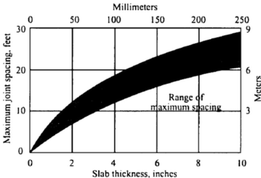
Figure 4.8 Suggested range of maximum spacing to be used together with the subgrade drag equation (Wire Reinforcement Institute, Inc., 2003).
