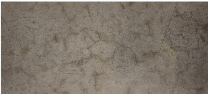
*Figure 5.10 Deviating area showing crazing for object 1.*
