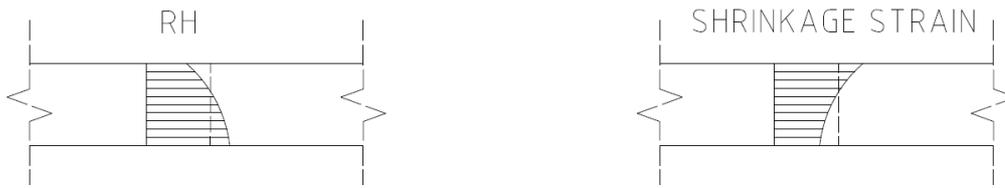
Figure 3.7 Distribution of RH and drying shrinkage strain in a slab section.
