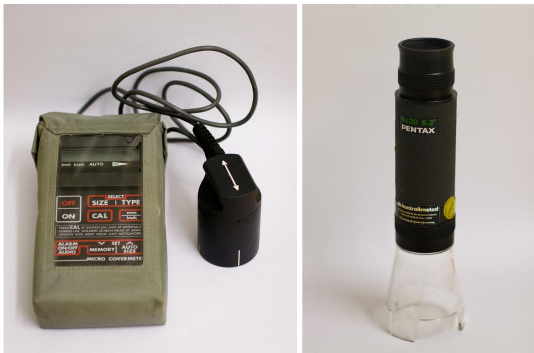
Figure 5.1 Cover meter and crack width microscope used for measurements.
