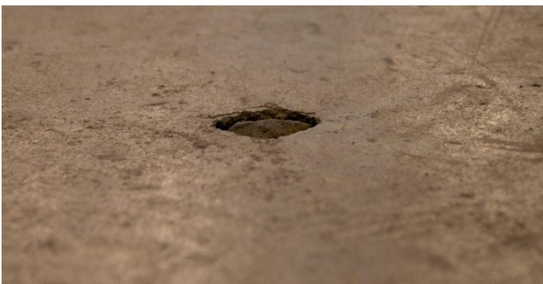
*Figure 5.11 Aggregate exposed in surface of object 1.*
