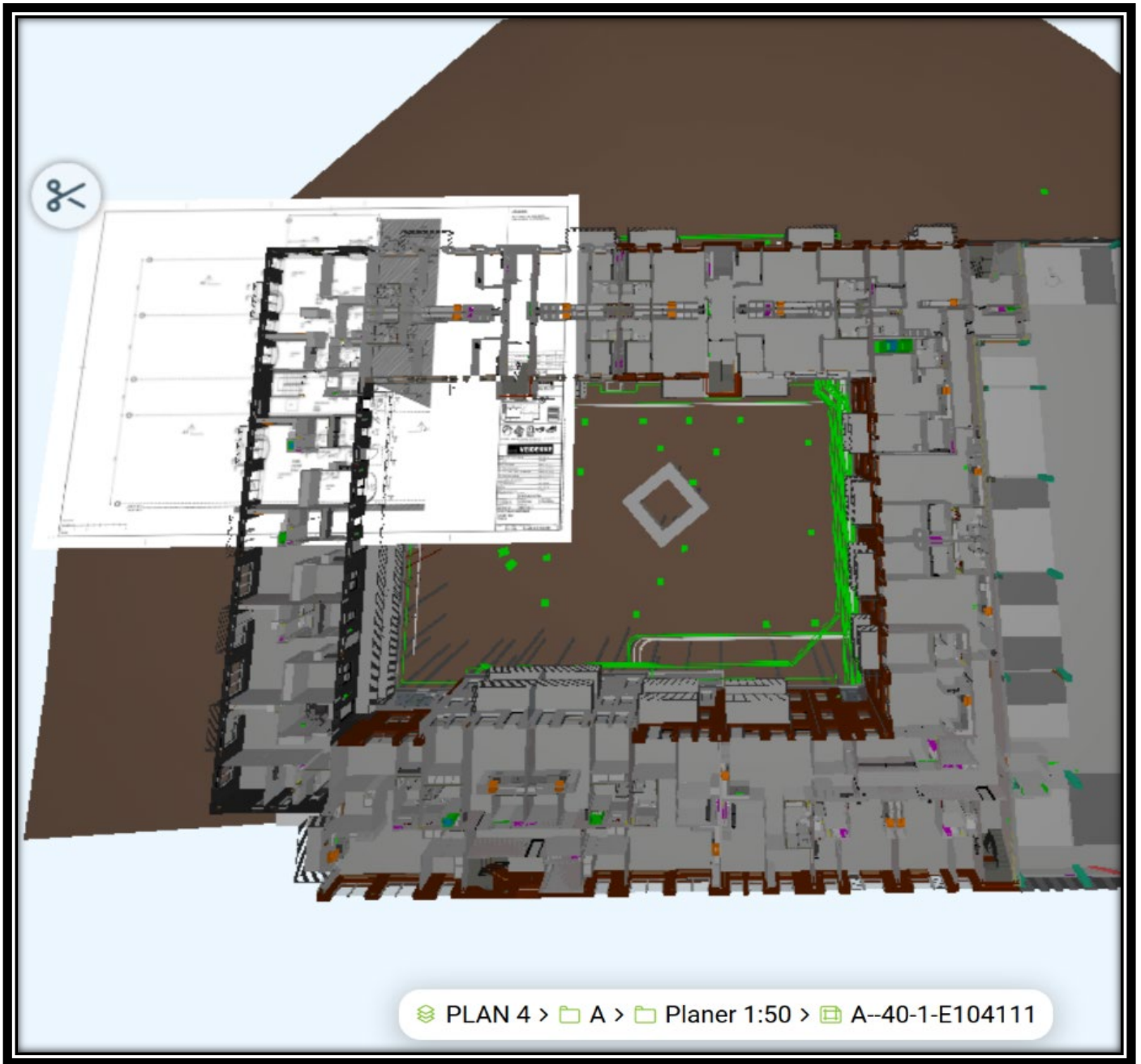
Figure 9 – a 3D model plane cut with underlying plane drawing for one of the sections.
