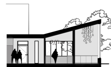
7 A tall glazed door in the entrance to expose the next space. Close-situated mullions in the office for a private feeling but with a view of the square
