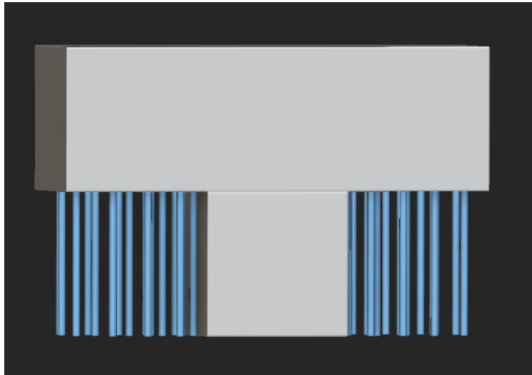
Figure 11: A part (in white) with support structure (in blue)
