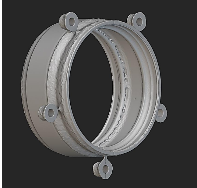
Figure 19: Resulting design from topology optimization for 5 ears
