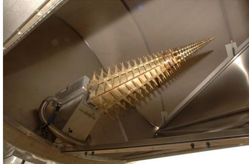
Figure 3.1.: The Allen Telescope Array feed [18].
