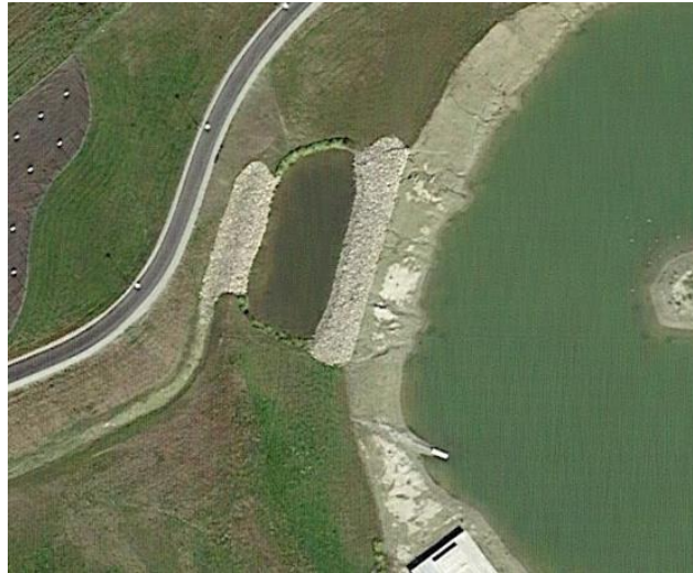
Figure 4-7 Rip-rap for energy dissipation upstream of Kunskapsdammen's forebay, Lund.
