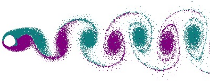
Figure 3.12: Kármán vortex street created by a cylindrical object where the flow on opposite sides of the object is given different colors, showing that the vortices are shed from alternating sides of the object (Wikipedia contributors, 2025).
