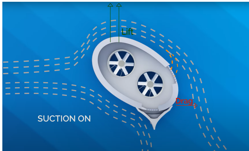
Figure 1.3: Aerodynamic operation of the bound4blue suction sail concept (bound4blue, 2025).
