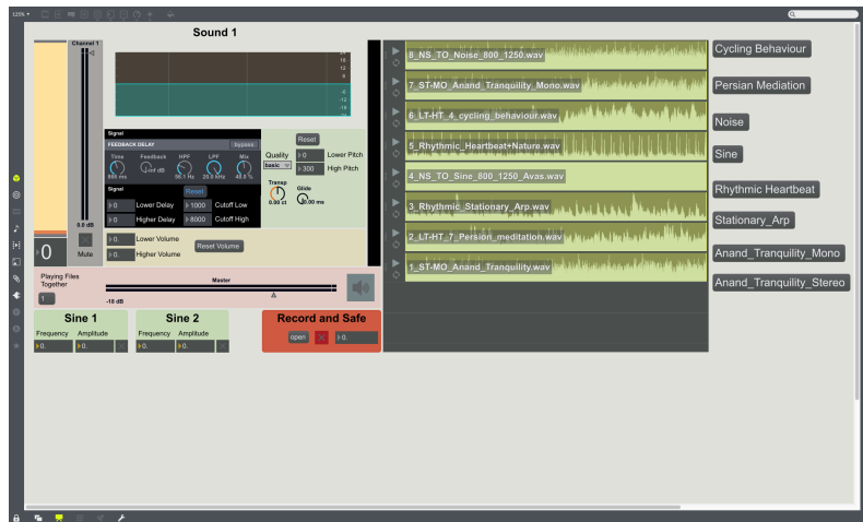
Figure 5.3: The GUI build in MAX/MSP to control sounds manually and automatically with the vehicle.
