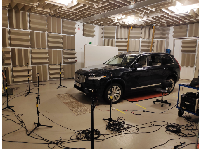
Figure 3.4: Semi-anechoic room with microphone setup.
