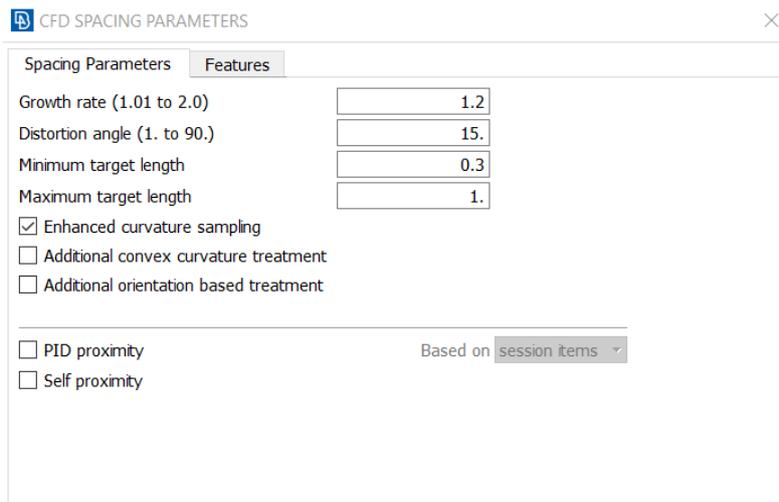
Figure 12 Surface mesh specification of the geometry
