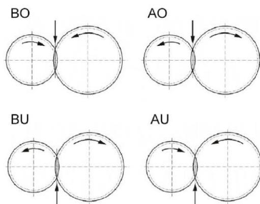
Figure 2 Different cases of spray lubrication [9]
