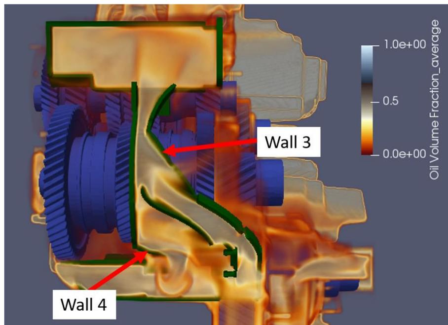
*Figure 24 Visualization of the flow to the container with the finished new part where wall 3 and 4 have been added after the results from previous simulation*
