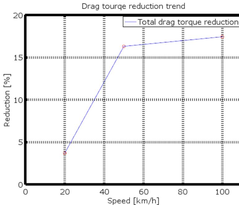
Figure 28 Trend of reduced drag torque with new part at three speeds
