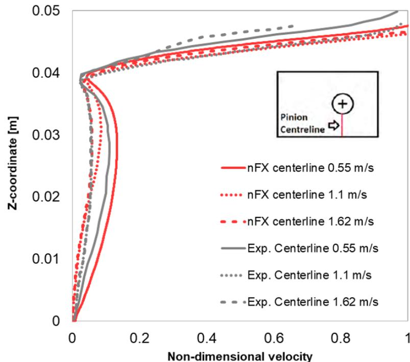
Figure 6 Velocity profile beneath pinion gear [4]
