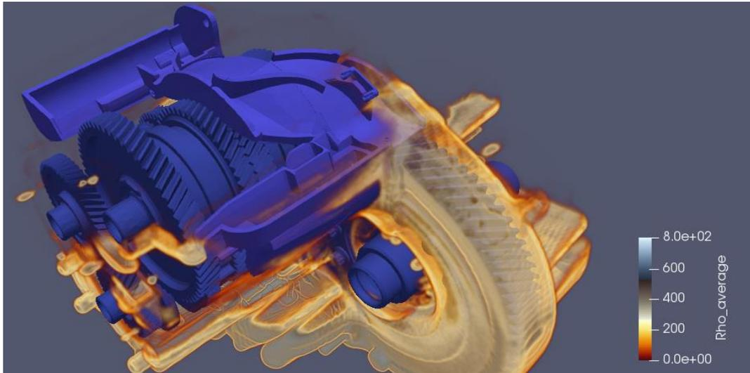
Figure 29 Overview of the gearbox 20km/h simulation results
