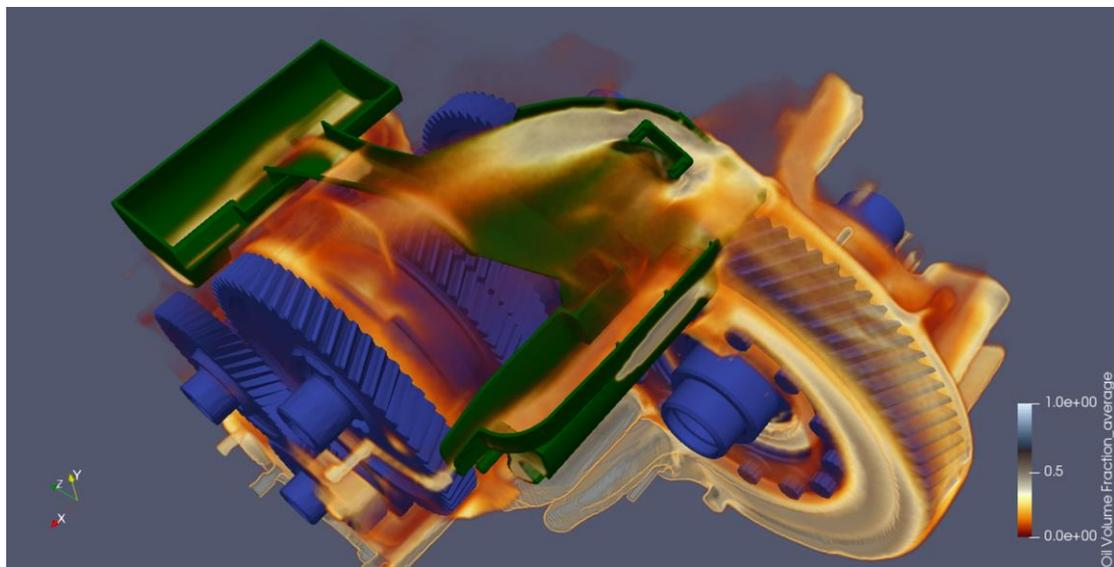
Figure 22 A first design of a new part that proves that the splash from the differential can be redirected
