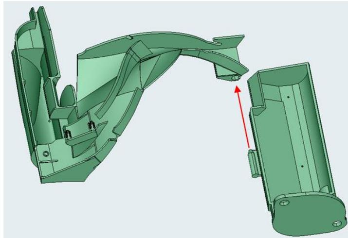
*Figure 37 Pin that slides into a slot while assembling the gearbox*
