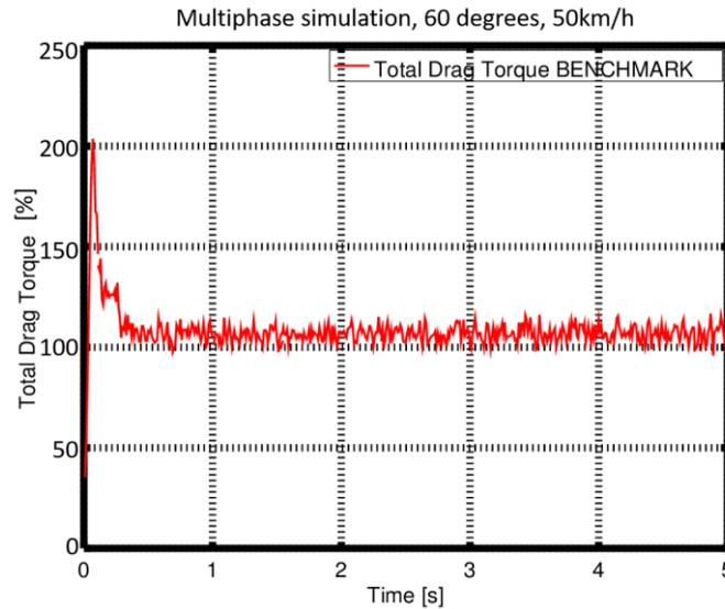
Figure 17 Total drag Torque of the benchmark simulation running for 5 seconds, values changed to percent due to confidentiality
