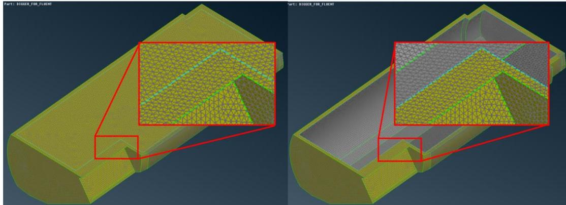
*Figure 11 Volume and surface meshed container*
