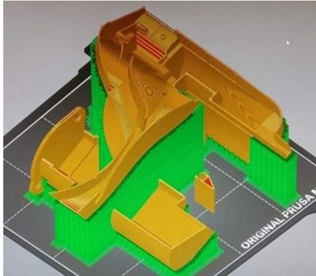
*Figure 38 Visualization of supports used in 3D-printing*
