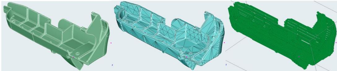
*Figure 8 Process from imported part to particles created*
