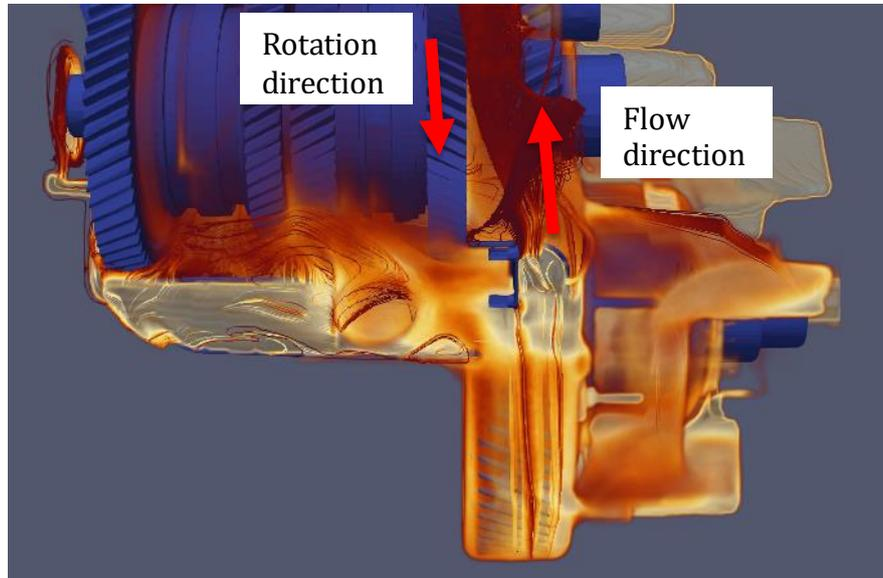
Figure 15 Top view of the gearbox with the differential in the bottom part of the figure transporting oil to the original trap above
