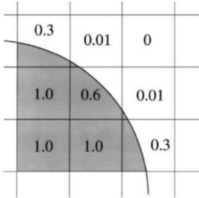
Figure 7 Representation of two immiscible fluids and interface [7]
