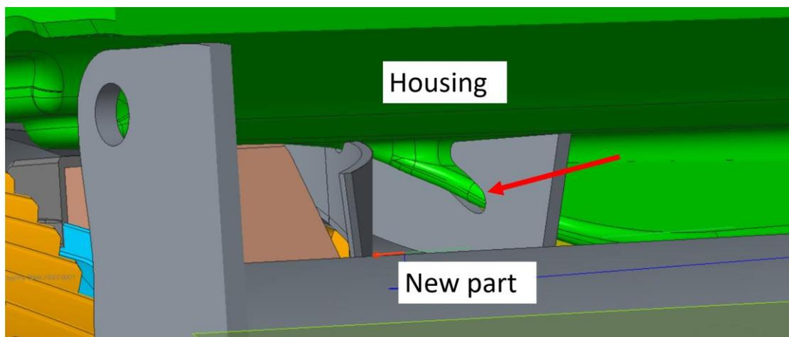
Figure 21 Example on how the new part was designed around obstacles, highlighted with an arrow
