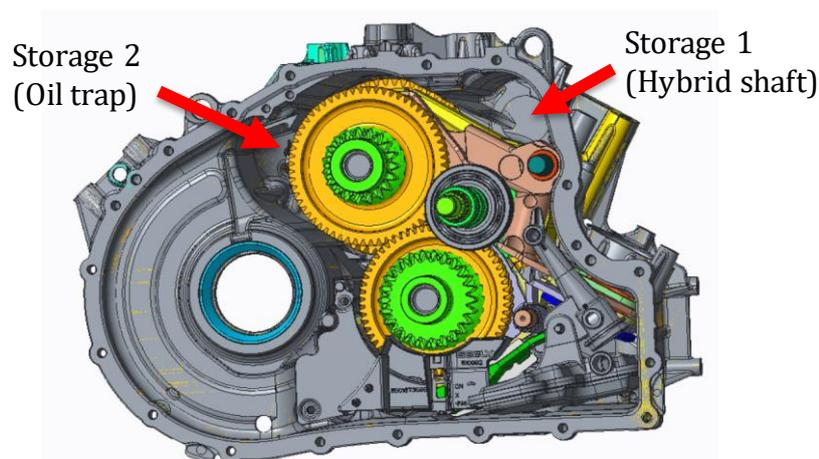
Figure 16 Two places where oil will be stored, here shown in a CAD picture with differential gear and original oil traps hidden
