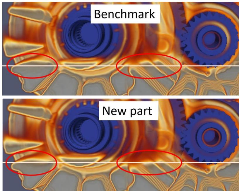
Figure 26 Circled in red, a comparison example between oil level in benchmark and new part case
