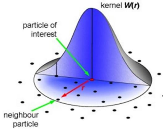
Figure 4 Gaussian Illustration of the Kernel function [6]
