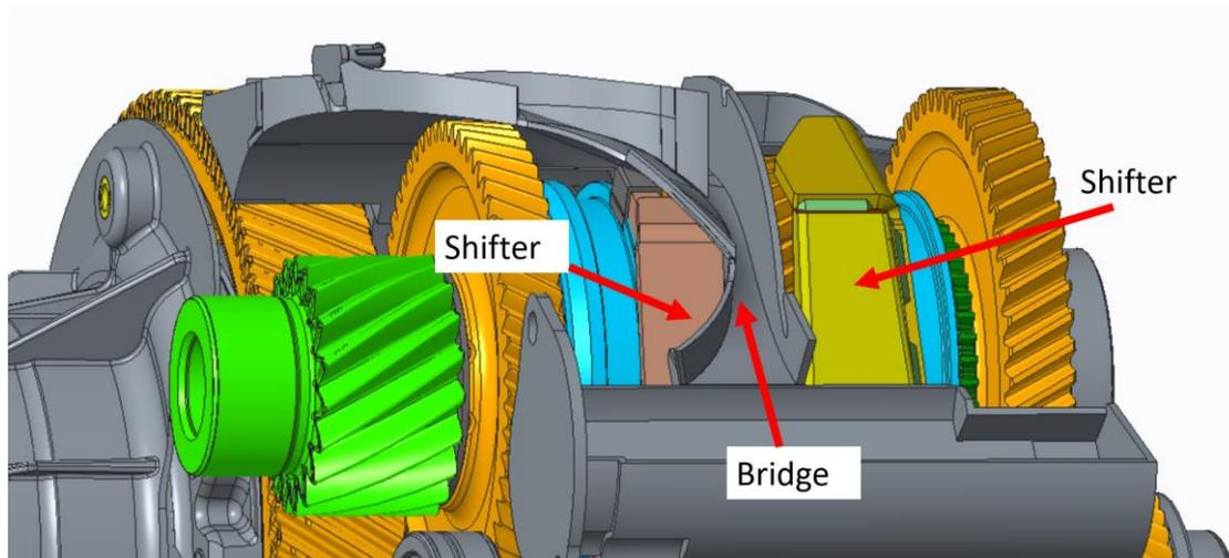
Figure 20 How the Bridge on the new part fits in between the shifters
