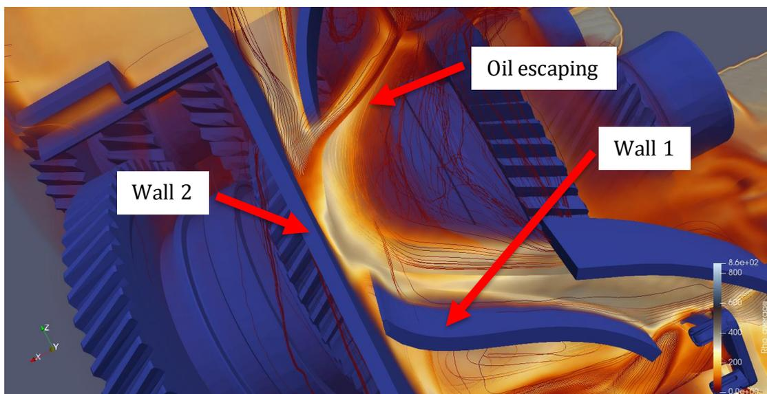
Figure 23 Second design of a new part with two added walls, wall 1 and wall 2
