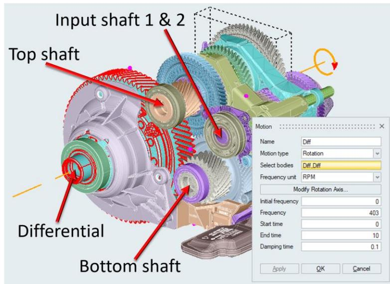
Figure 9 Internals of the 7DCT gearbox in Simlab with speed settings on differential gear and naming of the shafts used in the report
