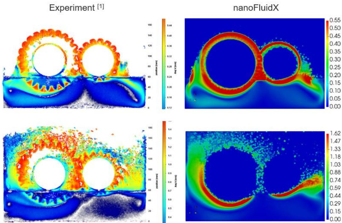
Figure 5 Particle image velocimetry study of two gears rotating in oil [4]
