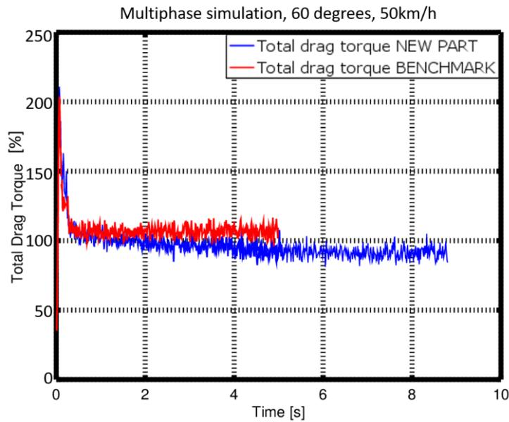
Figure 25 Total drag torque from new part and the benchmark at 50km/h
