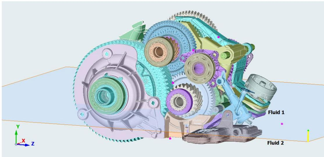
Figure 10 The plane that is defined in Simlab when creating particles of oil and air
