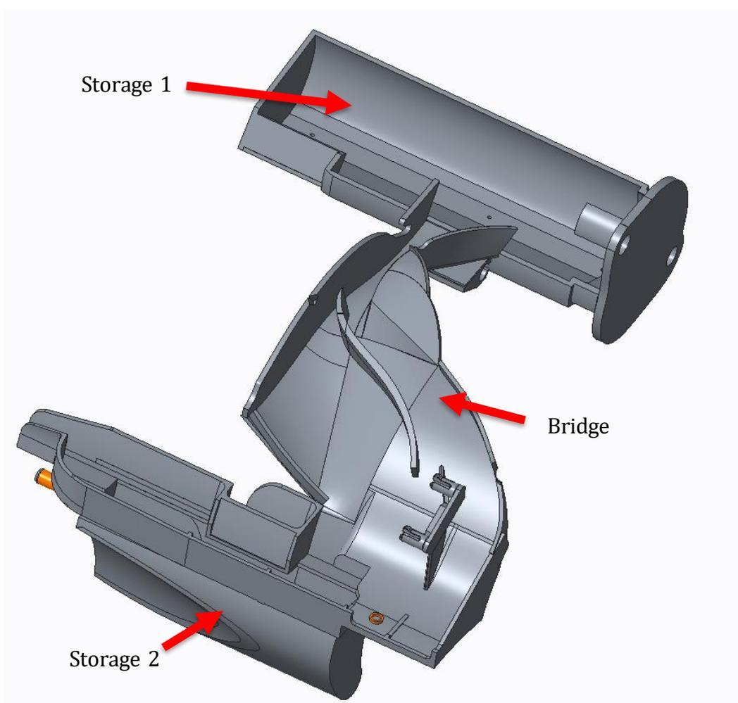
*Figure 19 New part that transports oil from the differential and collects it in two different places*
