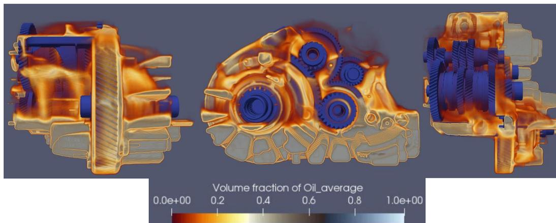
Figure 14 Overview of the gearbox benchmark simulation
