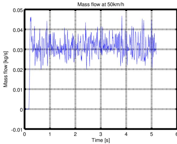
Figure 33 Mass flow entering the container at 50km/h
