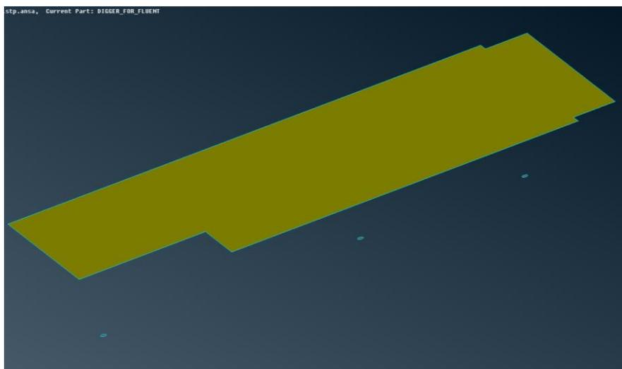
Figure 13 Pressure Outlet boundary surfaces – top and 3 outlet holes
