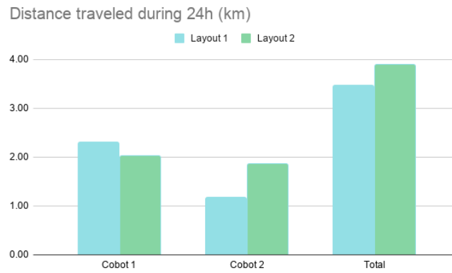
Figure 4.4: The distance in km travelled by each cobot during a 24h shift in TPS
