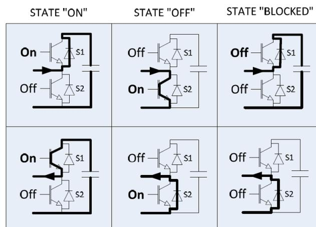
**Figure 2.8:** Operating state of half bridge cell [5]
