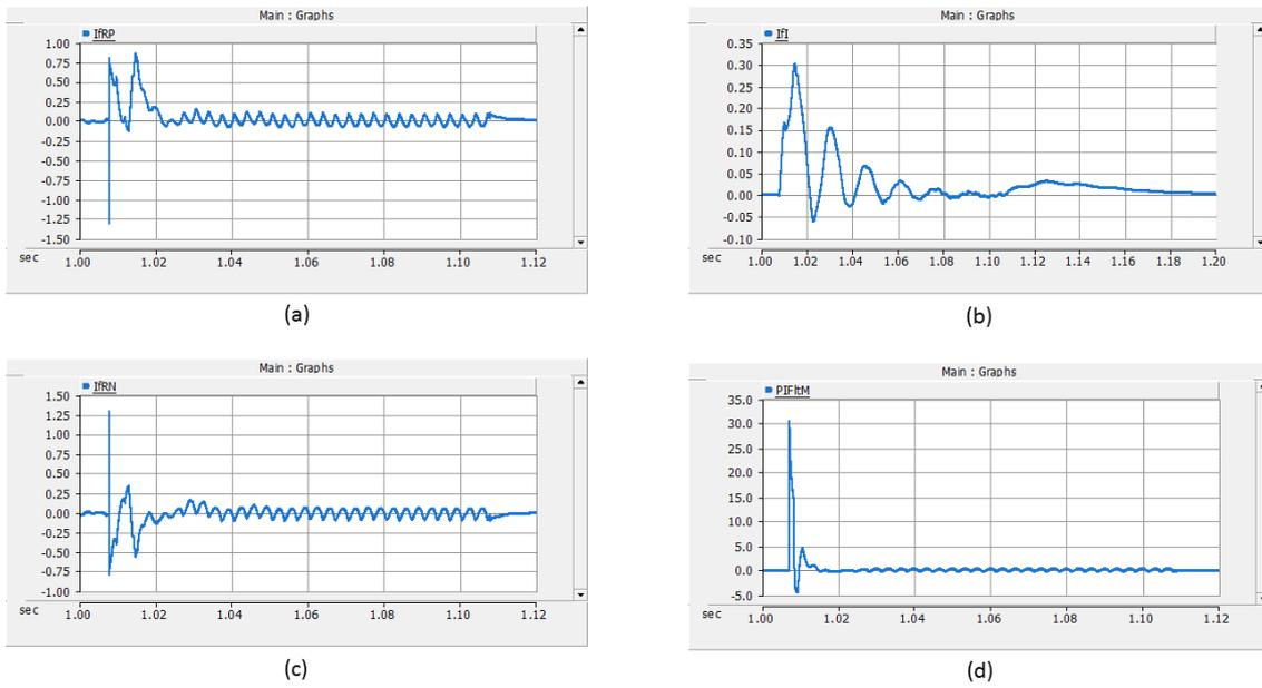
**Figure 4.7:** Simulation results for positive pole to ground fault at midpoint of the cable. (a) current through the rectifier side positive pole cable termination (peak = -1.29 kA), (b) current through the inverter side cable termination (peak = 0.302 kA), (c) current through the rectifier side negative pole cable termination (peak = 1.3 kA), (d) fault current due to positive pole to ground fault at midpoint of the cable (peak = 30.54 kA).
