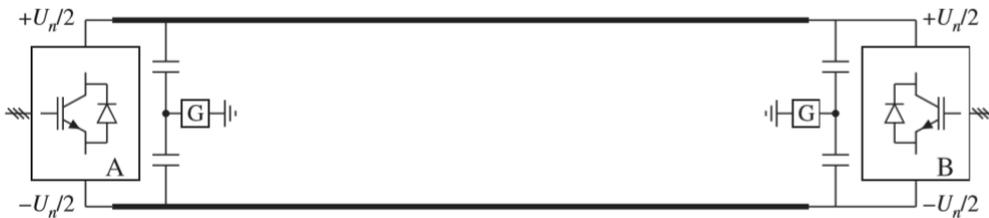
**Figure 2.2:** Symmetrical monopolar configuration [13]
