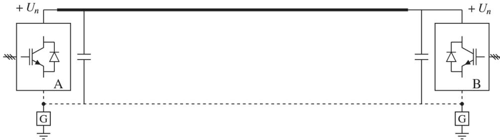
**Figure 2.1:** Asymmetrical monopolar configuration [13]
