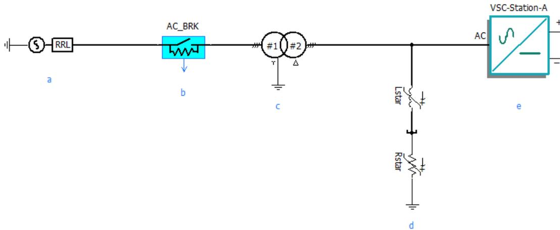
**Figure 3.1:** AC side model in PSCAD. a) AC grid, b) AC breaker, c) transformer, d) star point reactor and e) converter station
