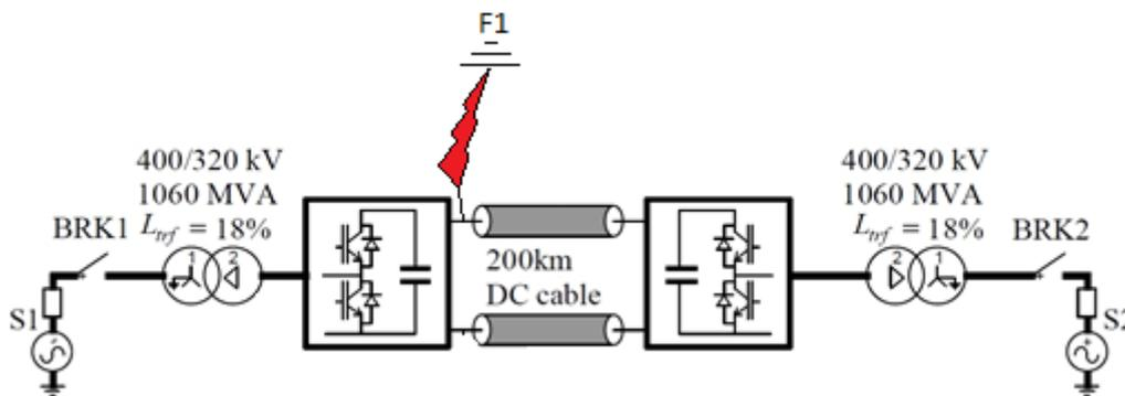
**Figure 4.2:** Positive pole to ground fault location in the symmetrical monopolar MMC VSC-HVDC system
