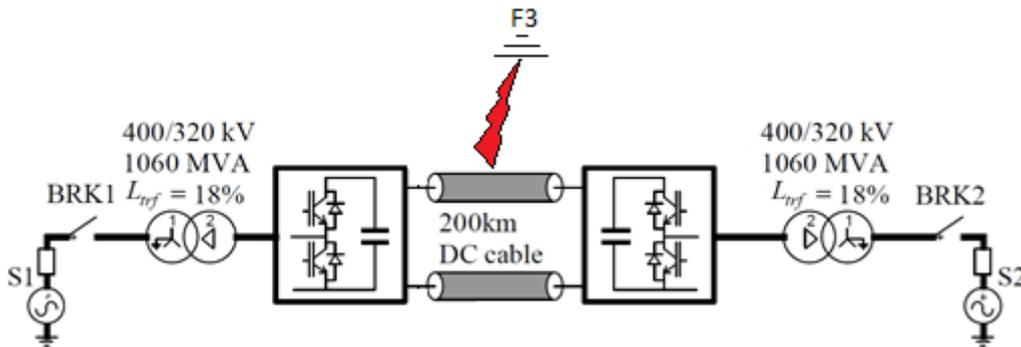
**Figure 4.6:** Positive pole to ground fault location in the symmetrical monopolar MMC VSC-HVDC system
