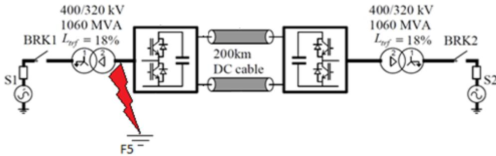
**Figure 4.12:** Single line to ground fault location in the symmetrical monopolar MMC VSC-HVDC system
