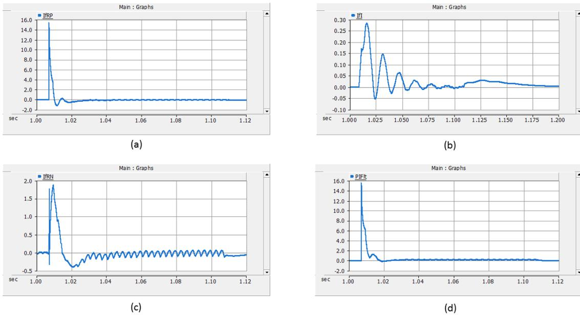
**Figure 4.3:** Simulation results for positive pole to ground fault at the DC terminals. (a) current through the rectifier side positive pole cable termination (peak = 15.4 kA), (b) current through the inverter side cable termination (peak = 0.28 kA), (c) current through the rectifier side negative pole cable termination (peak = 1.86 kA), (d) fault current due to positive pole to ground fault at the DC terminal of the converter station (peak = 15.5 kA).
