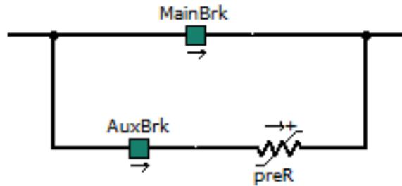
**Figure 3.2:** AC breaker model in PSCAD
