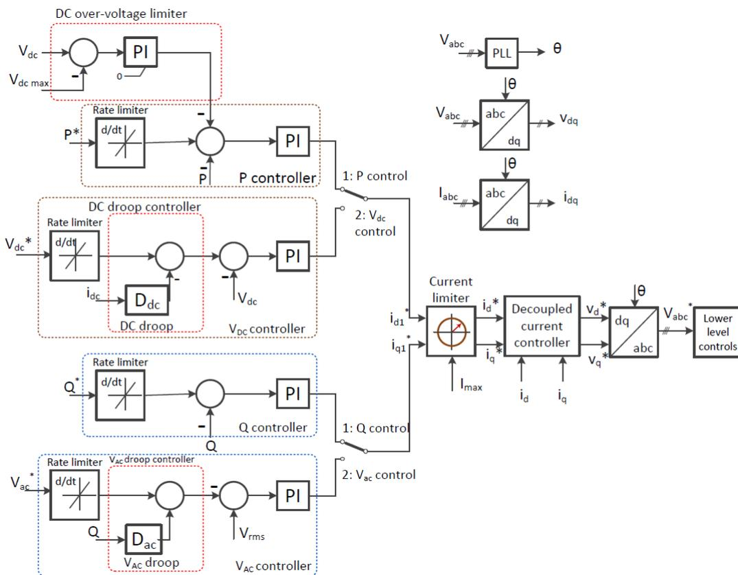
**Figure 2.6:** Upper level control configuration for non-islanded operation [5].
