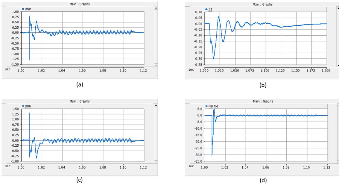
**Figure 4.10:** Simulation results for negative pole to ground fault at midpoint of the cable. (a) current through the rectifier side positive pole cable termination (peak = -1.3 kA), (b) current through the inverter side cable termination (peak = -0.302 kA), (c) current through the rectifier side negative pole cable termination (peak = 1.289 kA), (d) fault current due to negative pole to ground fault at midpoint of the cable (peak = -30.54 kA).
