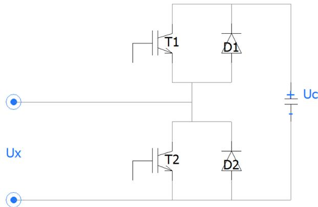
**Figure 2.7:** Half bridge converter topology
