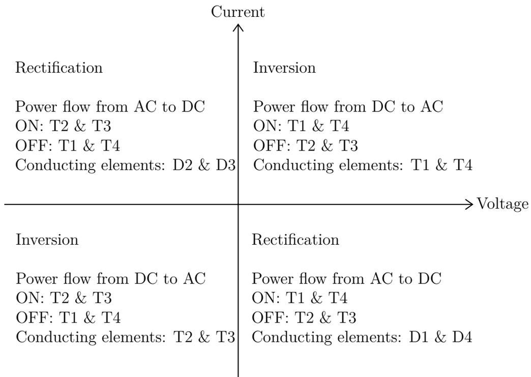
**Figure 2.10:** Four quadrant operation of full bridge or H bridge module
