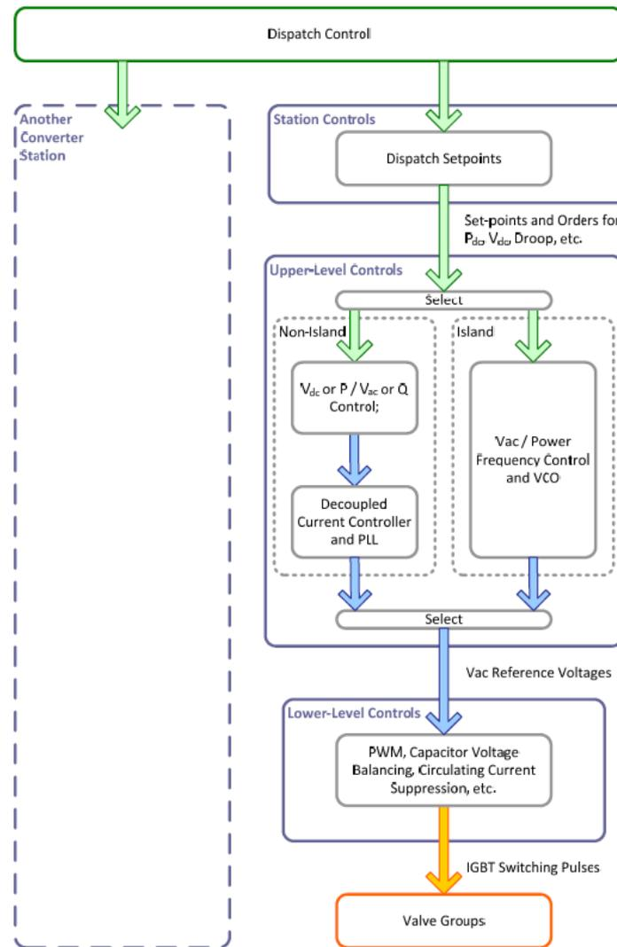
**Figure 2.5:** Generic control system hierarchy of VSC-HVDC converter [5]. Recommended for multi-terminal systems; indicated here for representative purposes
