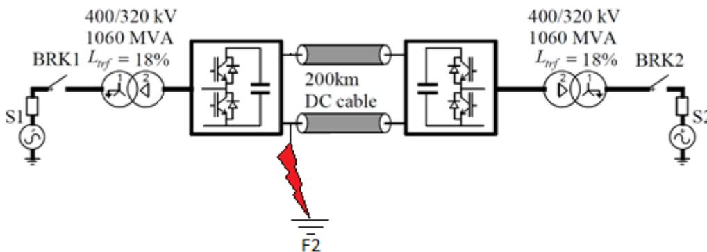
**Figure 4.4:** Negative pole to ground fault location in the symmetrical monopolar MMC VSC-HVDC system
