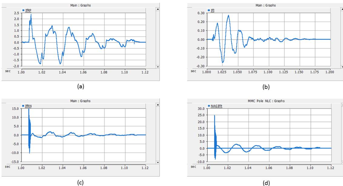
**Figure 4.17:** Simulation results for negative arm to ground fault at internal of the converter. (a) current through the rectifier side positive pole cable termination (peak = 2.337 kA), (b) current through the inverter side cable termination (peak = 0.27 kA), (c) current through the rectifier side negative pole cable termination (peak = 14.866 kA), (d) fault current due to negative arm to ground fault at internal of the converter (peak = 24.889 kA).
