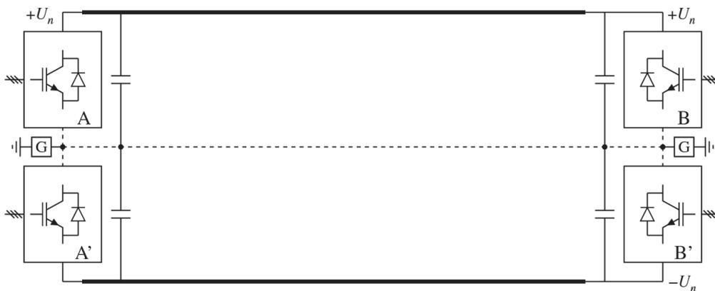
**Figure 2.3:** Bipolar configuration [13]
