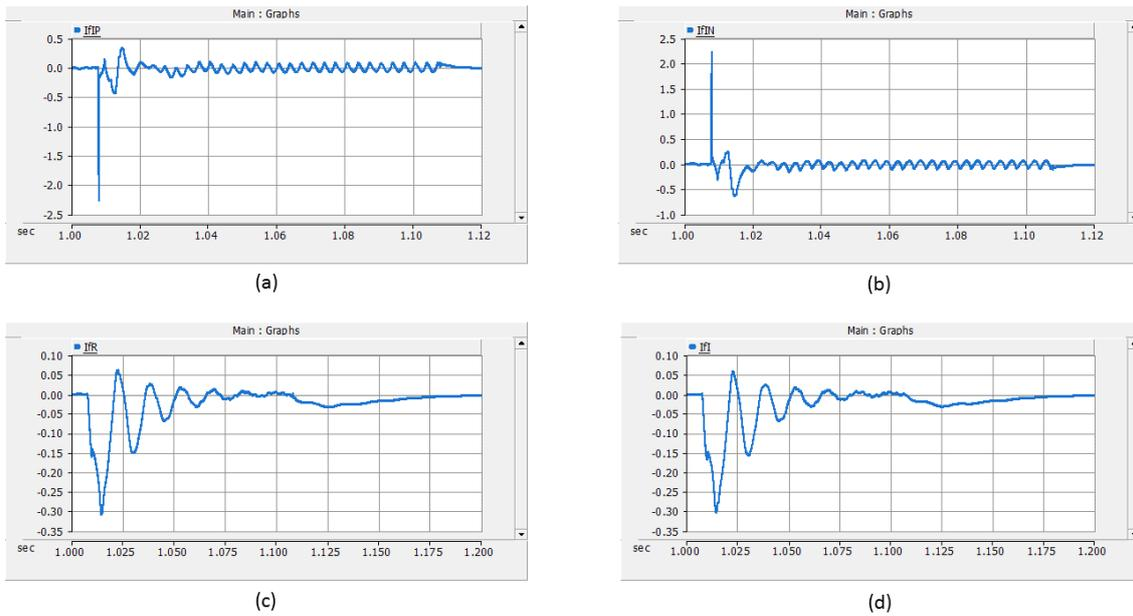
**Figure 4.11:** Simulation results for negative pole to ground fault at midpoint of the cable. (a) current through the inverter side positive pole cable termination (peak = -2.252 kA), (b) current through the inverter side negative pole cable termination (peak = 2.226 kA), (c) current through the rectifier side cable termination (peak = -0.307 kA), (d) current through the inverter side cable termination (peak = -0.302 kA).
