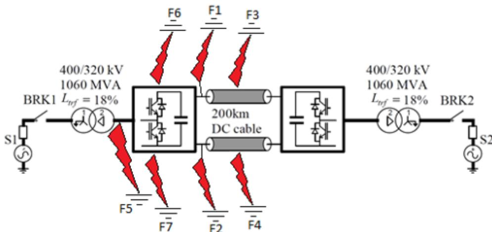
**Figure 4.1:** Fault location within the symmetrical monopolar MMC VSC-HVDC system
