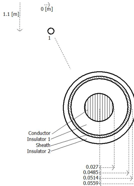
**Figure 3.3:** Land cable layers in PSCAD
