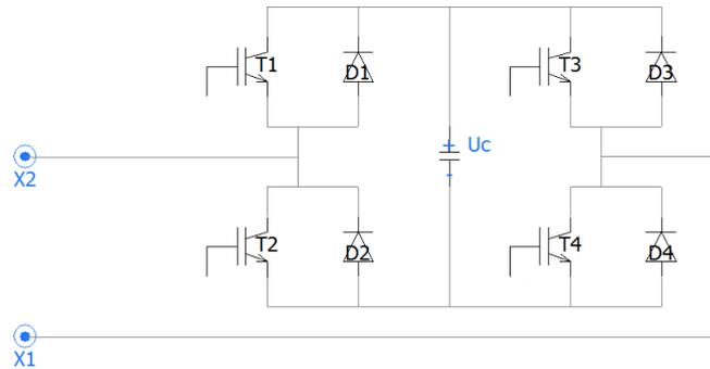
**Figure 2.9:** Full bridge or H bridge converter topology
