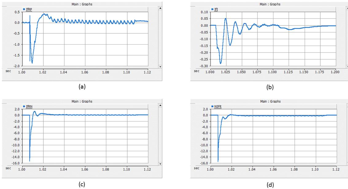
**Figure 4.5:** Simulation results for negative pole to ground fault at the DC terminals. (a) current through the rectifier side positive pole cable termination (peak = -1.87 kA), (b) current through the inverter side cable termination (peak = -0.28 kA), (c) current through the rectifier side negative pole cable termination (peak = -15.38 kA), (d) fault current due to negative pole to ground fault at the DC terminal of the converter station (peak = -15.5 kA).
