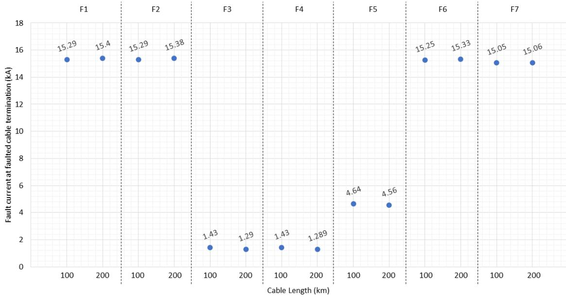
**Figure 4.19:** Graph showing the comparison between fault current at faulted cable termination and cable length
