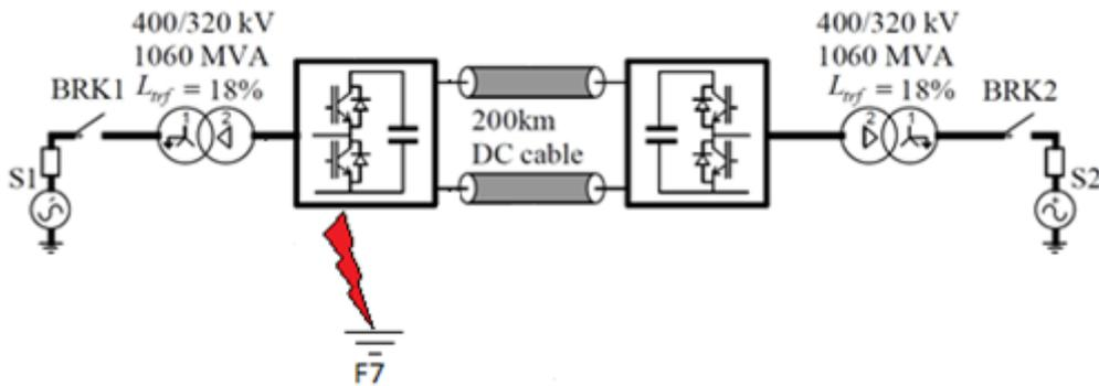
**Figure 4.16:** Negative arm to ground fault location in the symmetrical monopolar MMC VSC-HVDC system
