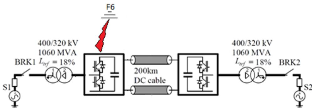
**Figure 4.14:** Positive arm to ground fault location in the symmetrical monopolar MMC VSC-HVDC system
