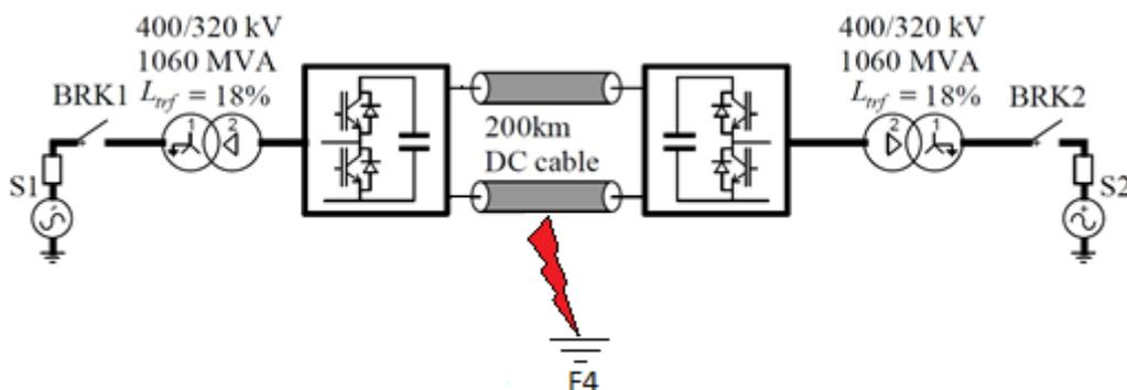
**Figure 4.9:** Negative pole to ground fault location in the symmetrical monopolar MMC VSC-HVDC system
