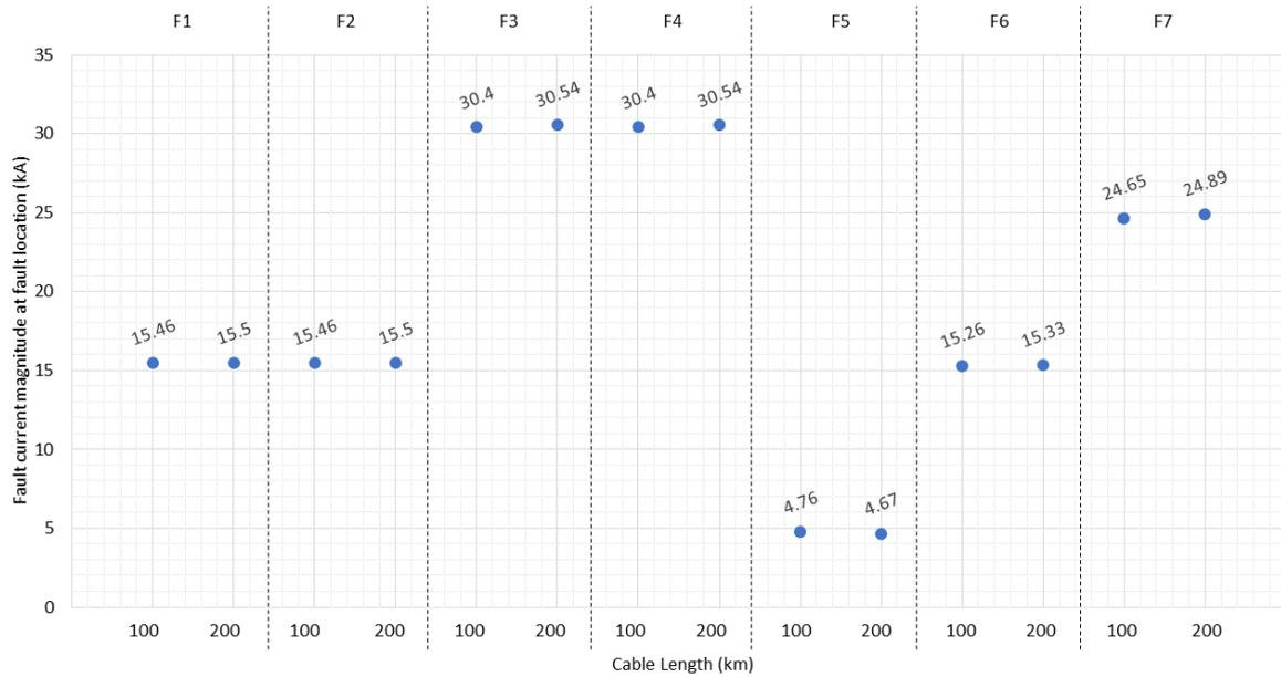
**Figure 4.18:** Graph showing the comparison between fault currents and cable length
