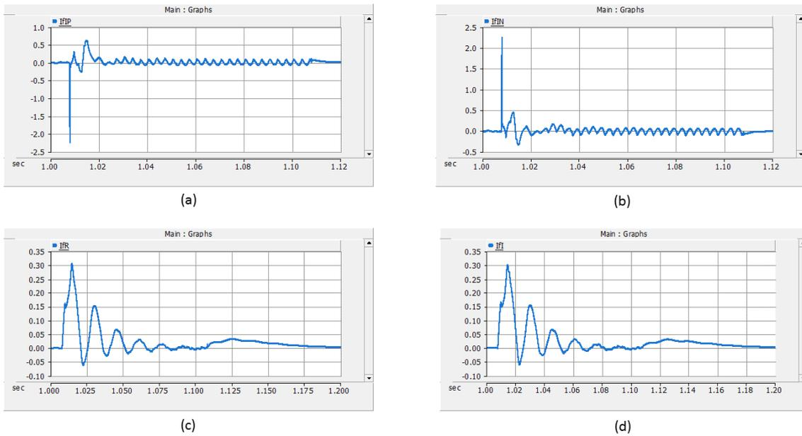
**Figure 4.8:** Simulation results for positive pole to ground fault at midpoint of the cable. (a) current through the inverter side positive pole cable termination (peak = -2.226 kA), (b) current through the inverter side negative pole cable termination (peak = 2.253 kA), (c) current through the rectifier side cable termination (peak = 0.305 kA), (d) current through the inverter side cable termination (peak = 0.302 kA).
