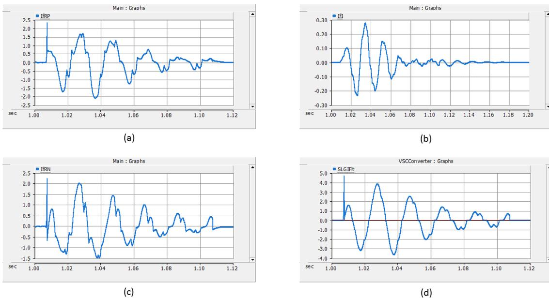
**Figure 4.13:** Simulation results for single line to ground fault at secondary side of the transformer. (a) current through the rectifier side positive pole cable termination (peak = 2.32 kA), (b) current through the inverter side cable termination (peak = 0.27 kA), (c) current through the rectifier side negative pole cable termination (peak = 2.24 kA), (d) fault current due to single line to ground fault at secondary side of the transformer (peak = 4.67 kA).
