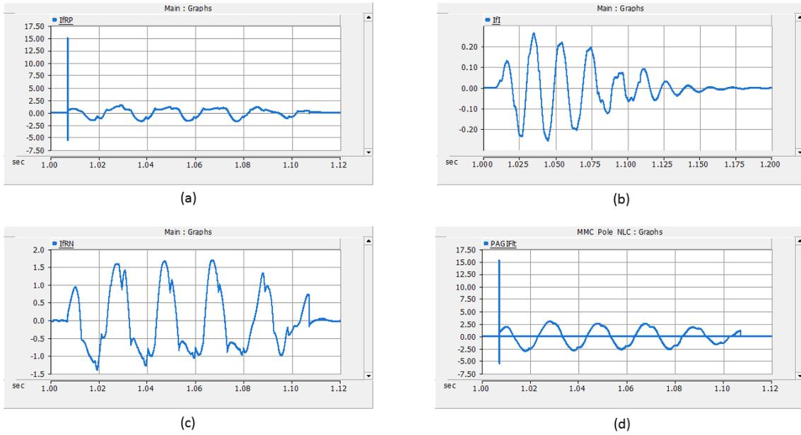
**Figure 4.15:** Simulation results for positive arm to ground fault at internal of the converter. (a) current through the rectifier side positive pole cable termination (peak = 15.143 kA), (b) current through the inverter side cable termination (peak = 0.26 kA), (c) current through the rectifier side negative pole cable termination (peak = 1.7 kA), (d) fault current due to positive arm to ground fault at internal of the converter (peak = 15.336 kA).
