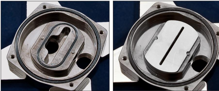
Fig. 5-6: Injection chamber and injection plate of the Koolance CPU-370, seen from below
