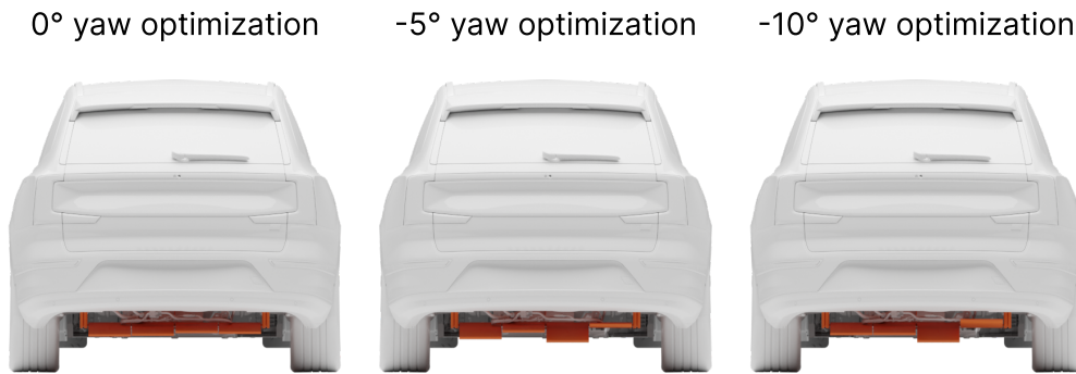
Figure 3.37: Visualization of the 4-dimensional optimized diffuser shape at different yaw values. In the scenario in which an active diffuser is implemented in a vehicle, its shape would change accordingly to best face side-wind conditions.
