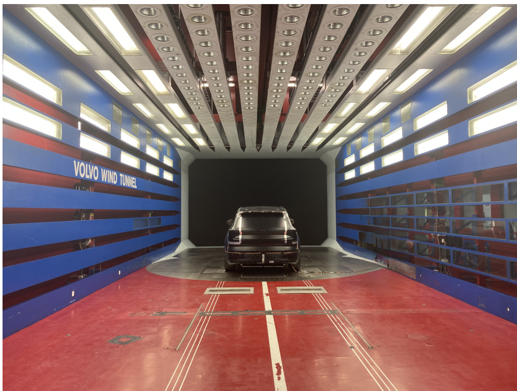
Figure 2.11: Clay car mounted on the wind tunnel balance.
