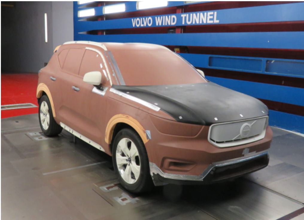
Figure 1.3: Example of clay car model. In the picture a Volvo XC40 is shown, located in the Volvo Cars wind tunnel facility.
