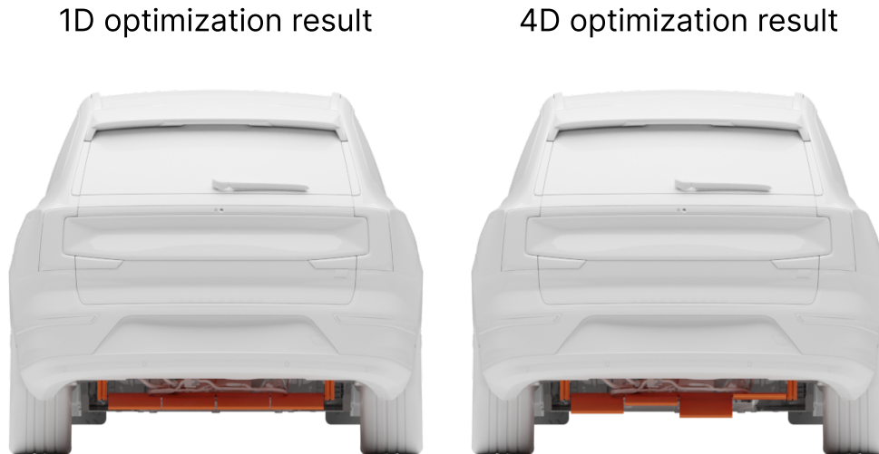
Figure 3.27: Visualization of the optimized diffuser shape obtained at -5^\circ yaw. On the left side, the outcome from 1-dimensional optimization is illustrated. On the right side, instead, the 4-dimensional optimization one.
