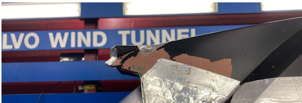
Figure 2.10: Roof kick added for the second clay car configuration
