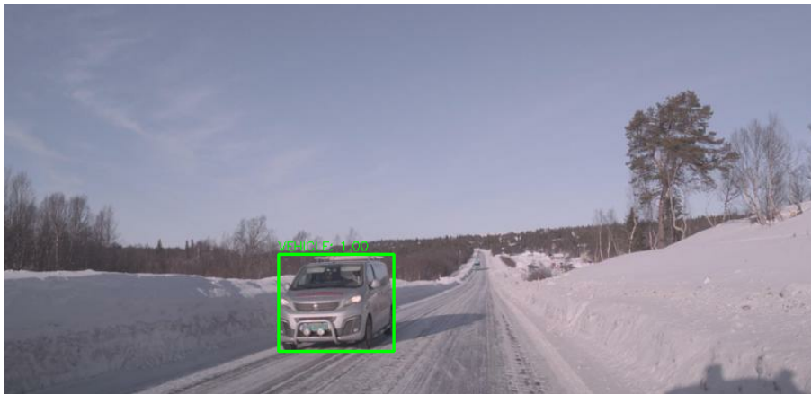
Figure 2.5: A training example from Zenseact Open Dataset (ZOD) 2 [30] where the 2d bounding box annotation has been overlaid onto the image.
