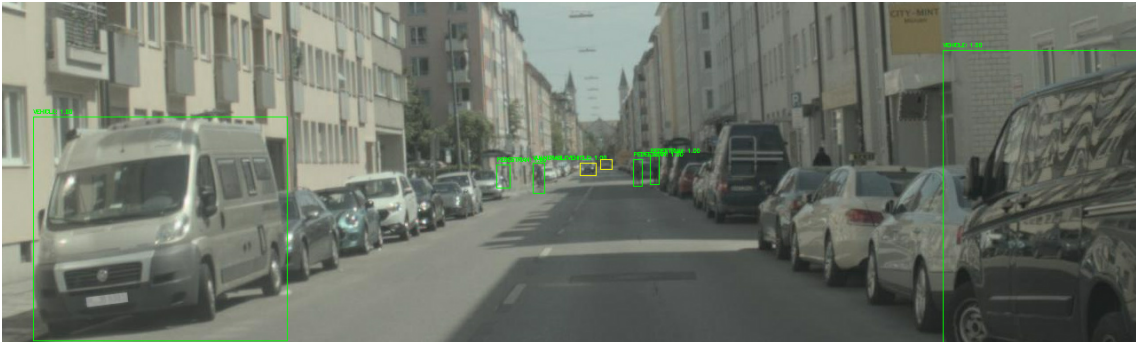
Figure C.1: An example of a mislabeled sample. Multiple vehicles have been left without a corresponding object annotation.
