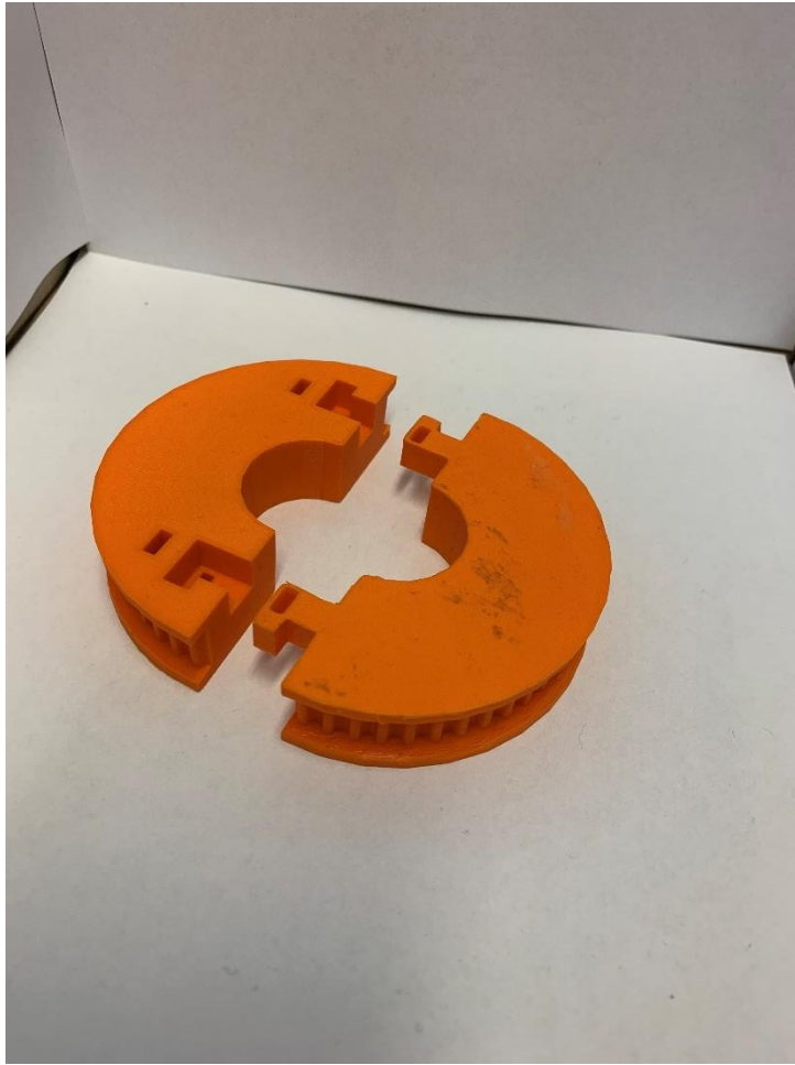
Final gear with integrated interlocking mechanism (separated)
