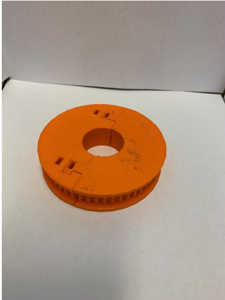
Final gear with integrated interlocking mechanism (interlocked)
