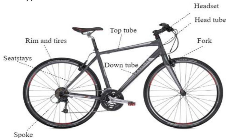
Figure 1 – Bicycle and its components
