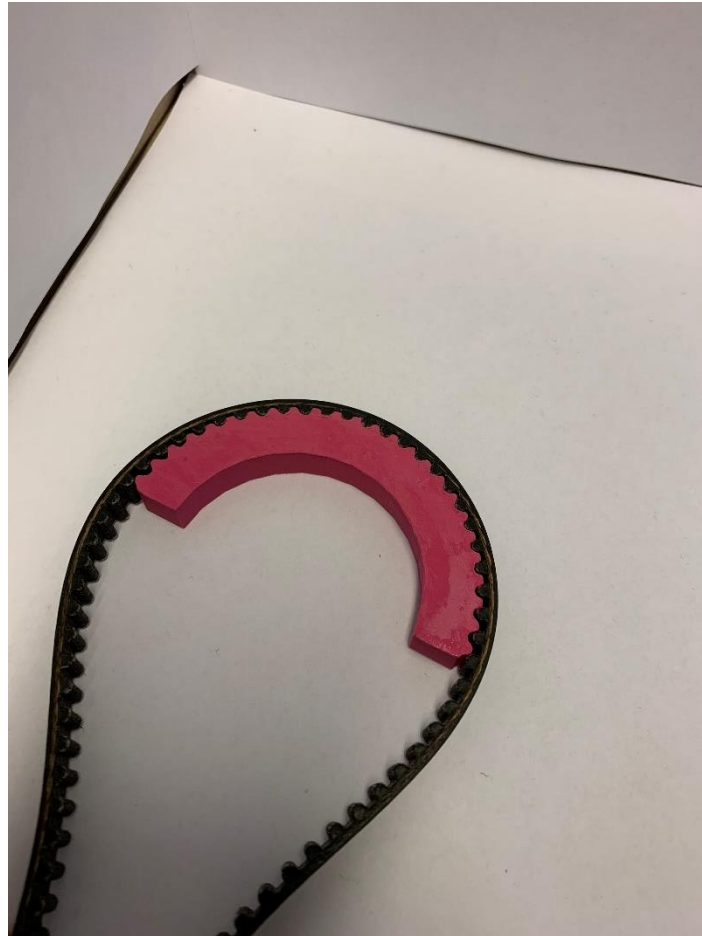
First successful gear prototype that matches the already existing timing belt
