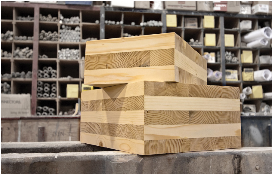
Figure 2.1: Cut of a three layer and five layer CLT element. "Cross laminated timber blocks" by ODF is licensed under CC BY 2.0.
