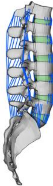
Figure 2. The new FE-model of the lumbar spine (L1-L5) developed by Iraeus et al. (2023), scaled to average male size to fit the SAFER HBM.
