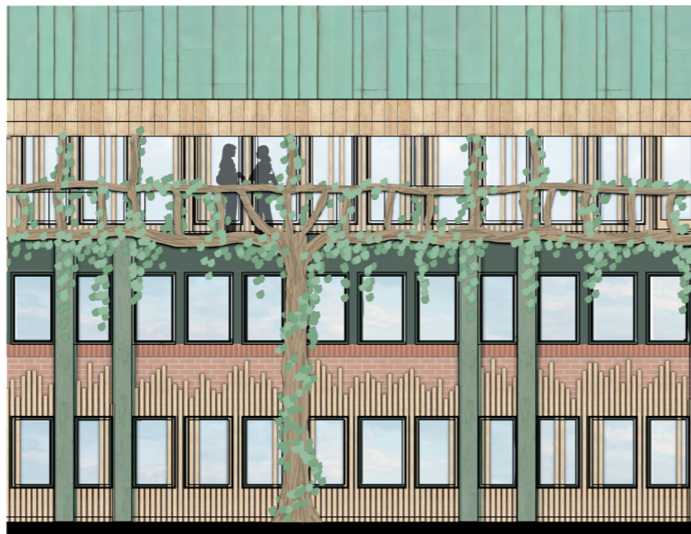
Figure 50: After facade showing dynamic wooden elements and tree-shaped pergola (1:100 A4).
