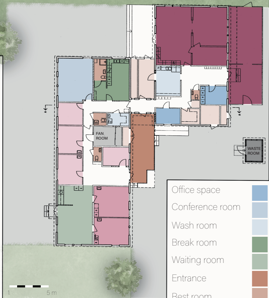
Figure 38: Family centre floor plan (1:300 A4).
