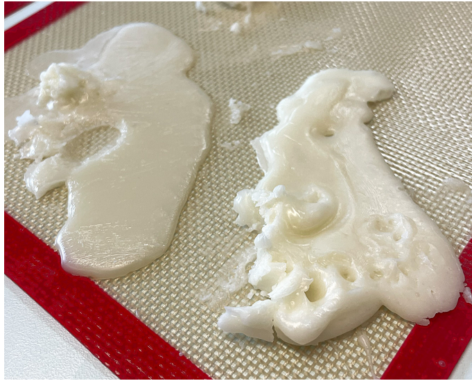
Figure C.1: Visual observation of bigel extruded at high speed. Due to the rapid extrusion, the material was deposited in a more liquid-like state, forming uneven "pools" that quickly solidified upon deposition.
