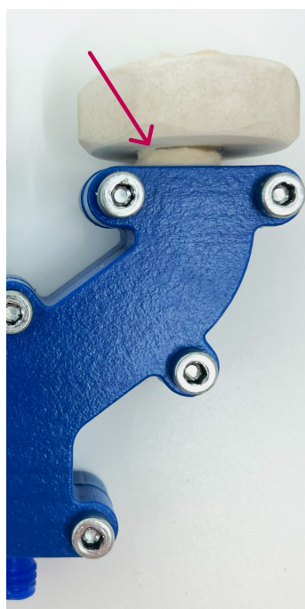
Figure D.4: Visual observation of leakage from the mixing module during extrusion of emulsion gel. The arrow indicates gel escaping at the cartridge connection point, suggesting that the material, due to its rheological properties, occasionally found alternative paths instead of exiting through the nozzle.
