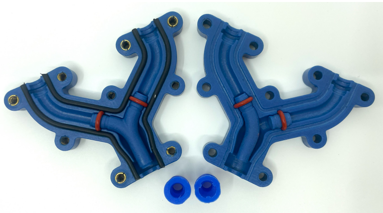
Figure 2.2: A prototype of the custom-made mixing module, constructed in plastic with interchangeable components. The left configuration illustrates the dual extrusion mode, where two materials are deposited side by side. The right configuration shows the coaxial extrusion mode, in which one material is extruded through a core surrounded by the second material.
