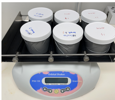
Figure 4.2: Acid leaching with inorganic acid and organic acid on orbital shaker.
