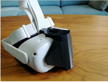
Figure 6.7: Top view of the holder attached to the Oculus Quest 2.
