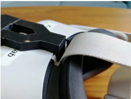
Figure 6.9: Top hook clutching the upper part of the Oculus Quest 2.
