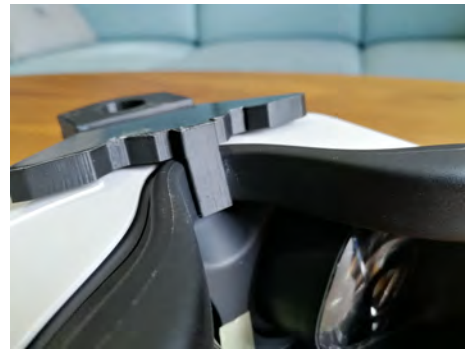
Figure 6.10: Bottom hook clutching the lower part of the Oculus Quest 2.
