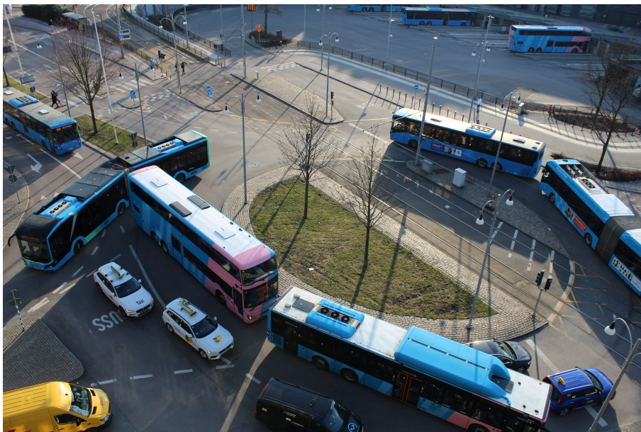
Figure 4.2: A gridlock caused by the vehicles in the roundabout blocking a bus trying to enter the bus lane
