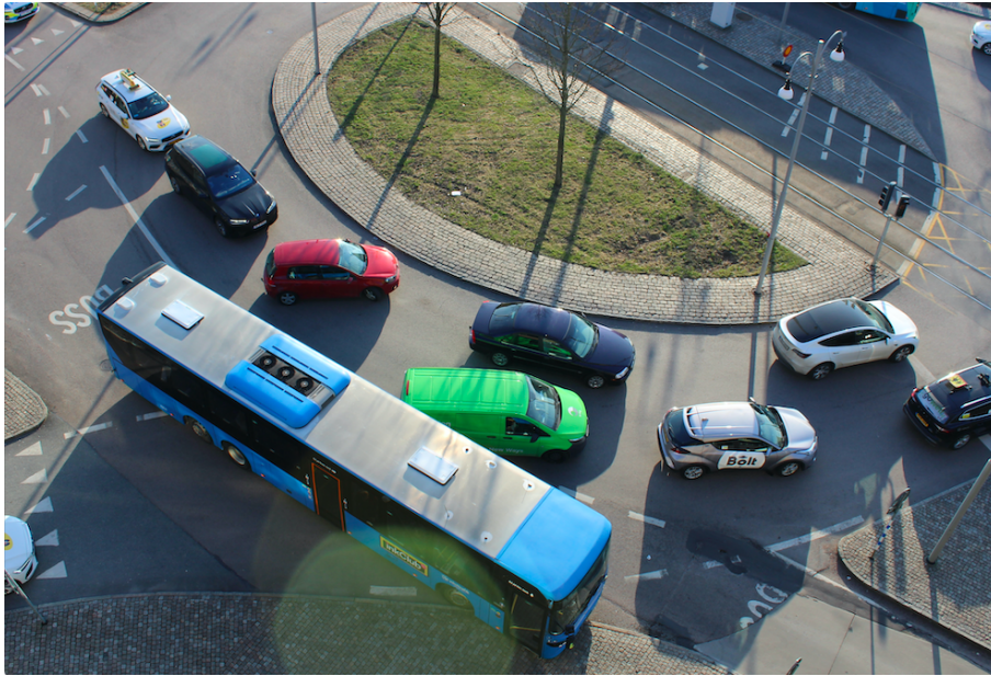
Figure 4.4: Cars wrongfully queuing in two lanes, blocking the bus from entering the dedicated bus lane
