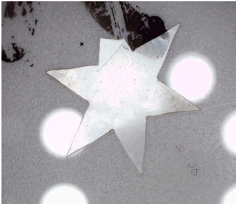
Sample 1 peltier module test for star with 0.4V and 0.2A(left) and 1V and 0.4A (right)
