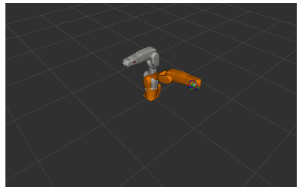
Figure 5.11: Displays robot before execution with the grey model being the current robot position and orange the selected goal state
