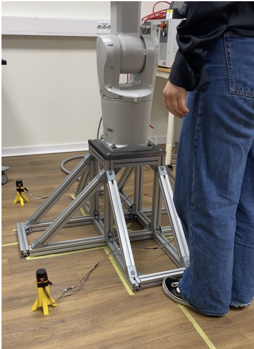
Figure 4.15: Demonstration of LEDs lighting up when a person breaches a security zone. The safety zones are here smaller than allowed due to demonstration purposes.
