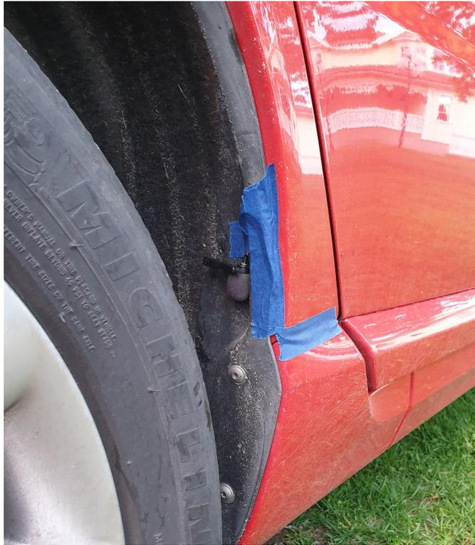
**Figure 3.1:** The placement of the microphone when collecting road noise for the road surface noise dataset.
