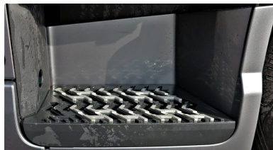
Figure 4.35: Image of the driver side instep of the truck after driving through the wading channel at speed v_2 during the test
