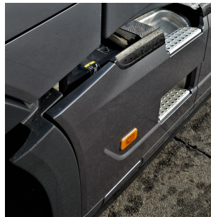
Figure 4.39: Image of the driver side side skirt of the truck after driving through the wading channel at speed v_1 during the test
