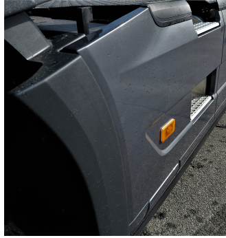
Figure 4.37: Image of the driver side side skirt of the truck after driving through the wading channel at speed v_1 during the test
