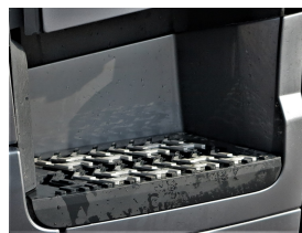
Figure 4.33: Image of the driver side instep of the truck after driving through the wading channel at speed v_1 during the test
