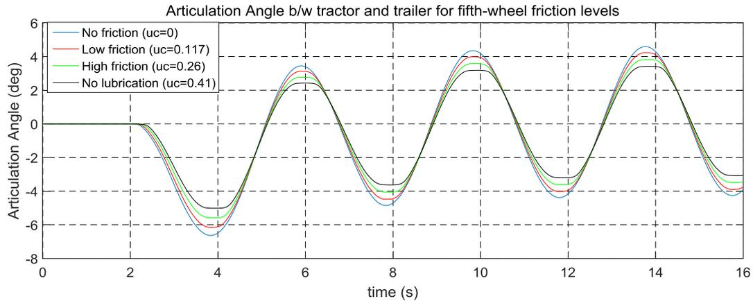
Figure 42 Articulation Angle for different levels of fifth-wheel friction
