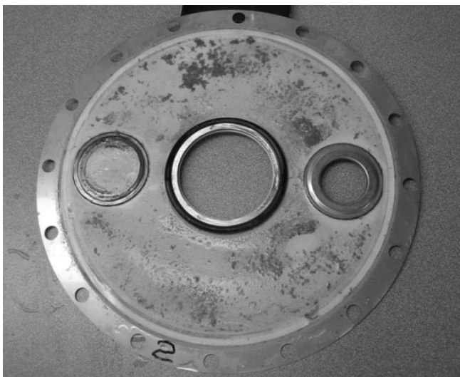
Figure 27. Most common appearance of the membranes.
