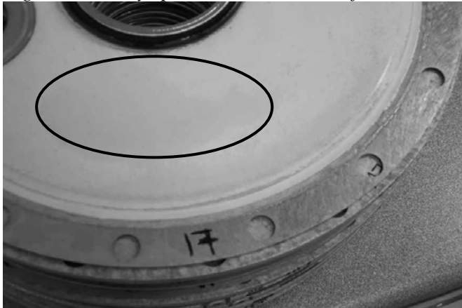
Figure 26. Turbulent zones give change in colour on membrane surface.
