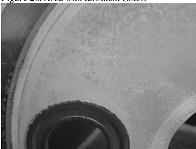
Figure 29. Fouling that is strongly bound to the surface.
