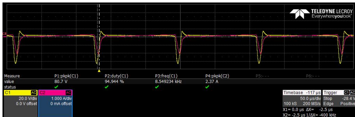
Figure 5.5: Voltage & current plot across the circular receiver coil 2 under normal operation between the Tx & Rx coils
