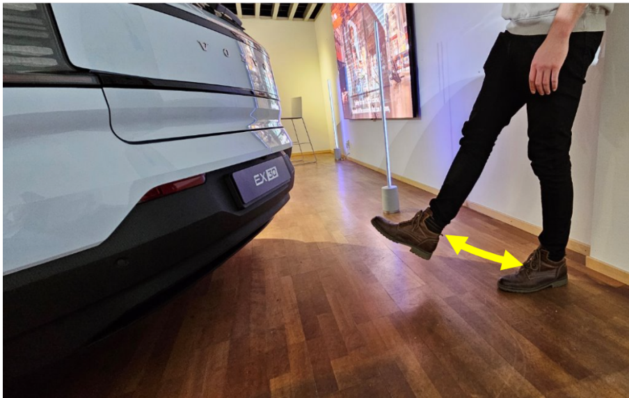
Figure 3.1: Illustration of the leg 'kick' gesture. Note that the distance between the starting position and the vehicle was roughly one meter.
