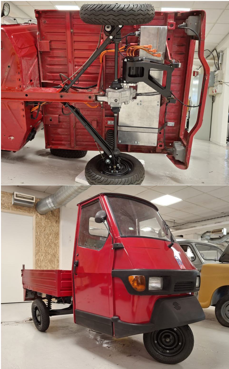
Figure 6.1: Installed Electric Conversion Kit
