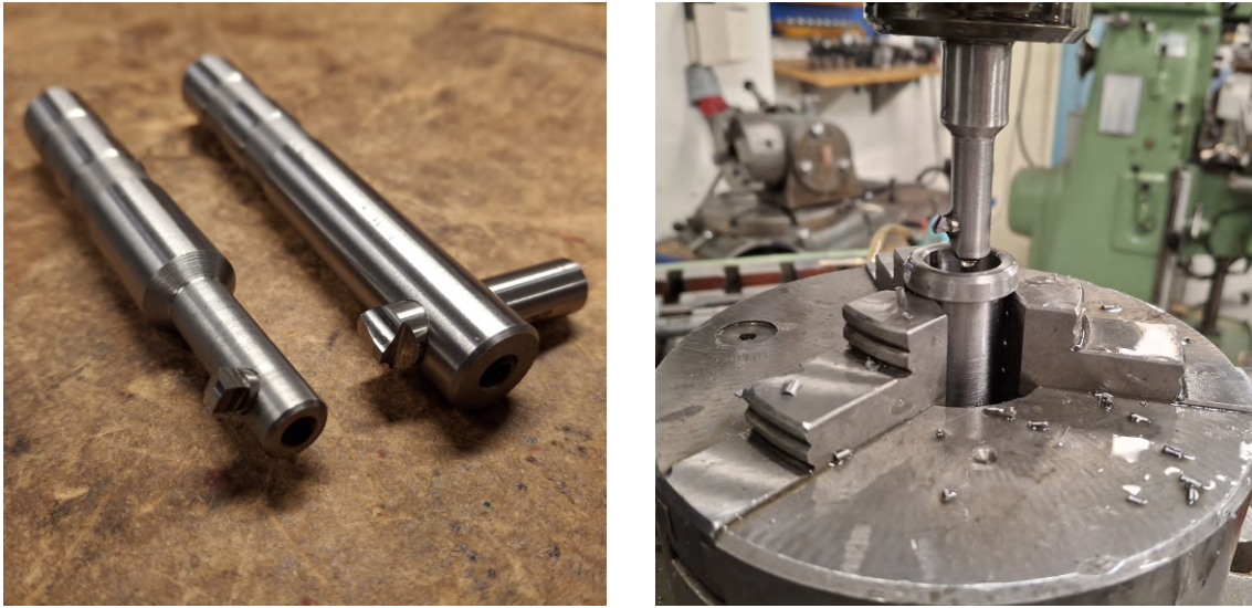
Figure 5.2: HSS Spline cutting tools and spline shaping Process
