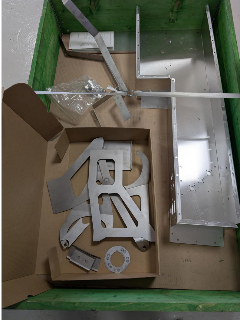
Figure 5.6: Laser cut and bent sheet metal parts
