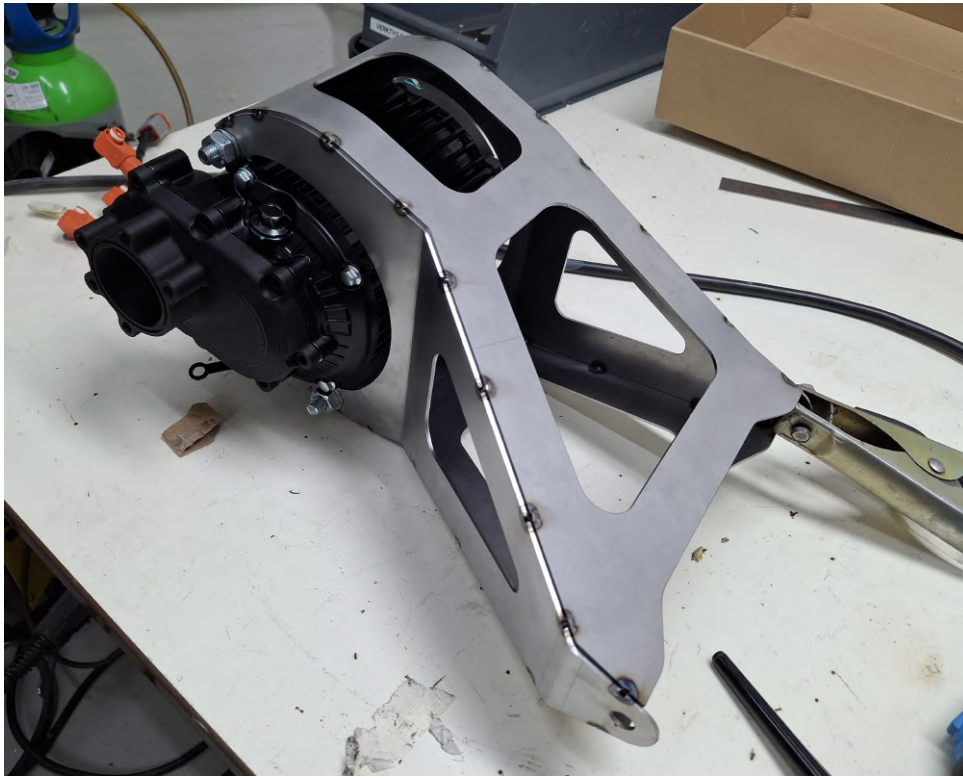
Figure 5.11: Spot welded motor mount
