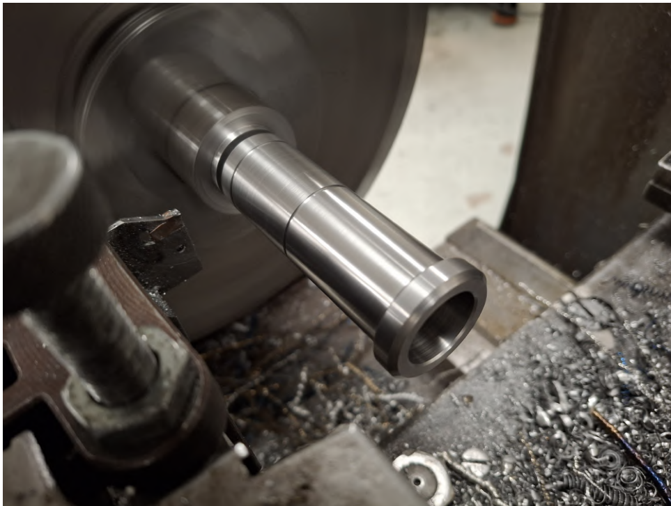
Figure 5.1: Spline shaft blank being turned in a lathe
