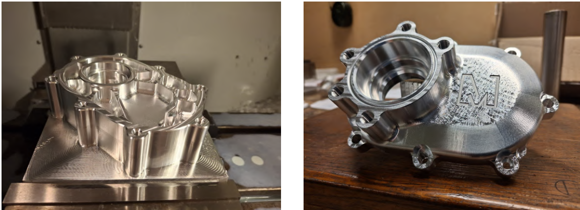
Figure 5.5: Motor to differential adapter
