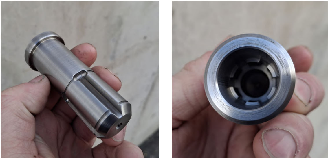
Figure 5.3: Spline shaft prior to heat treatment
