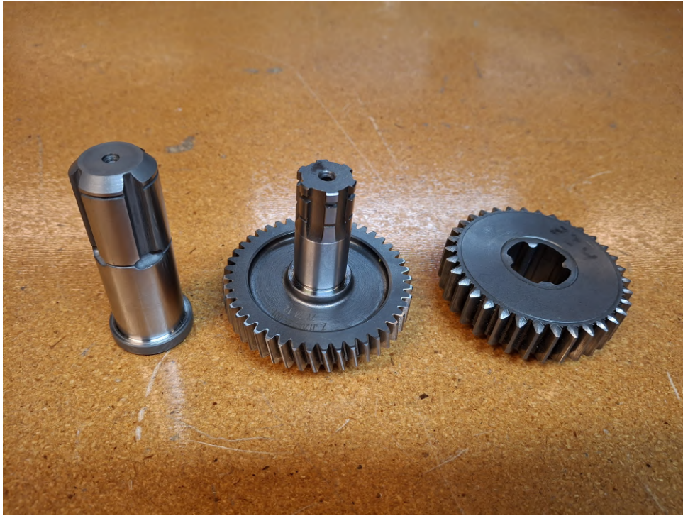
Figure 5.4: Spline shaft, motor output gear and final drive input gear
