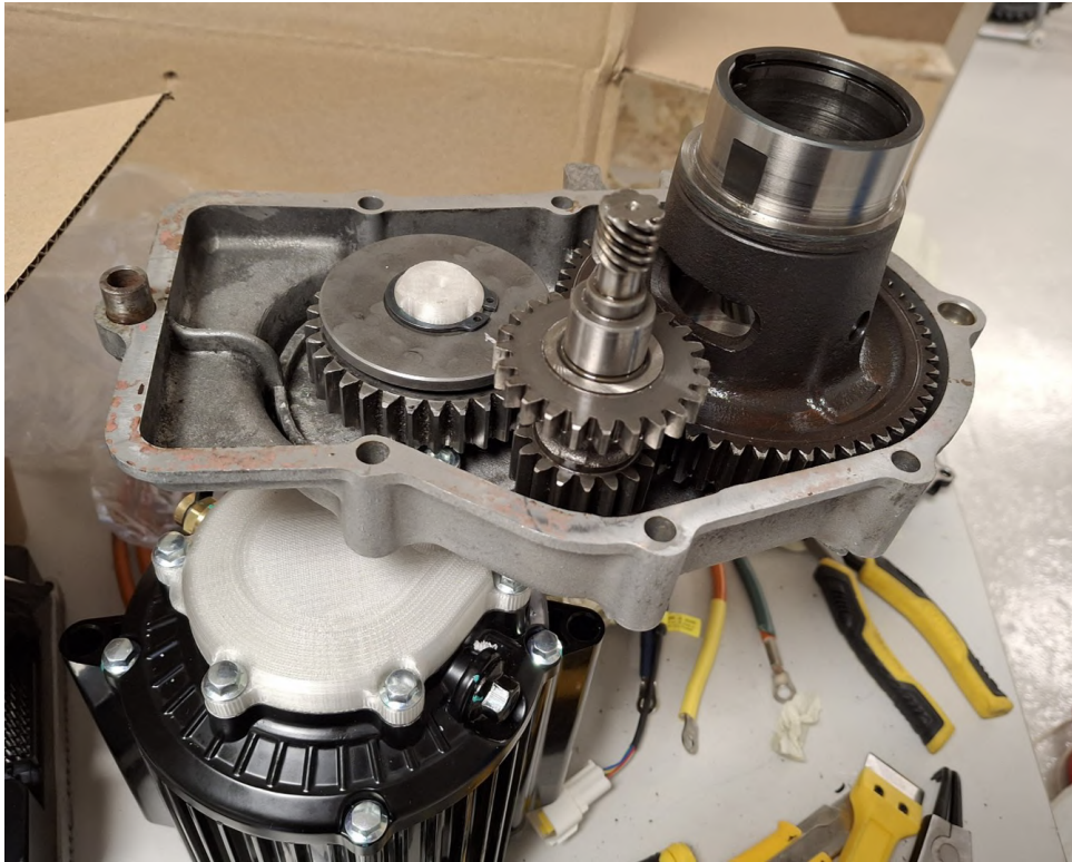
Figure 4.7: Motor and differential assembled with 3D-printed parts
