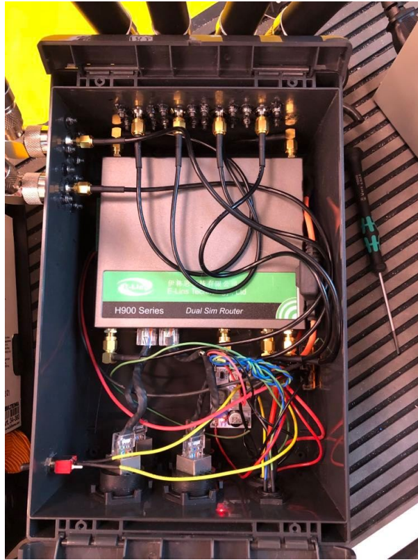
Figure 3.1: The internals of the SCU
